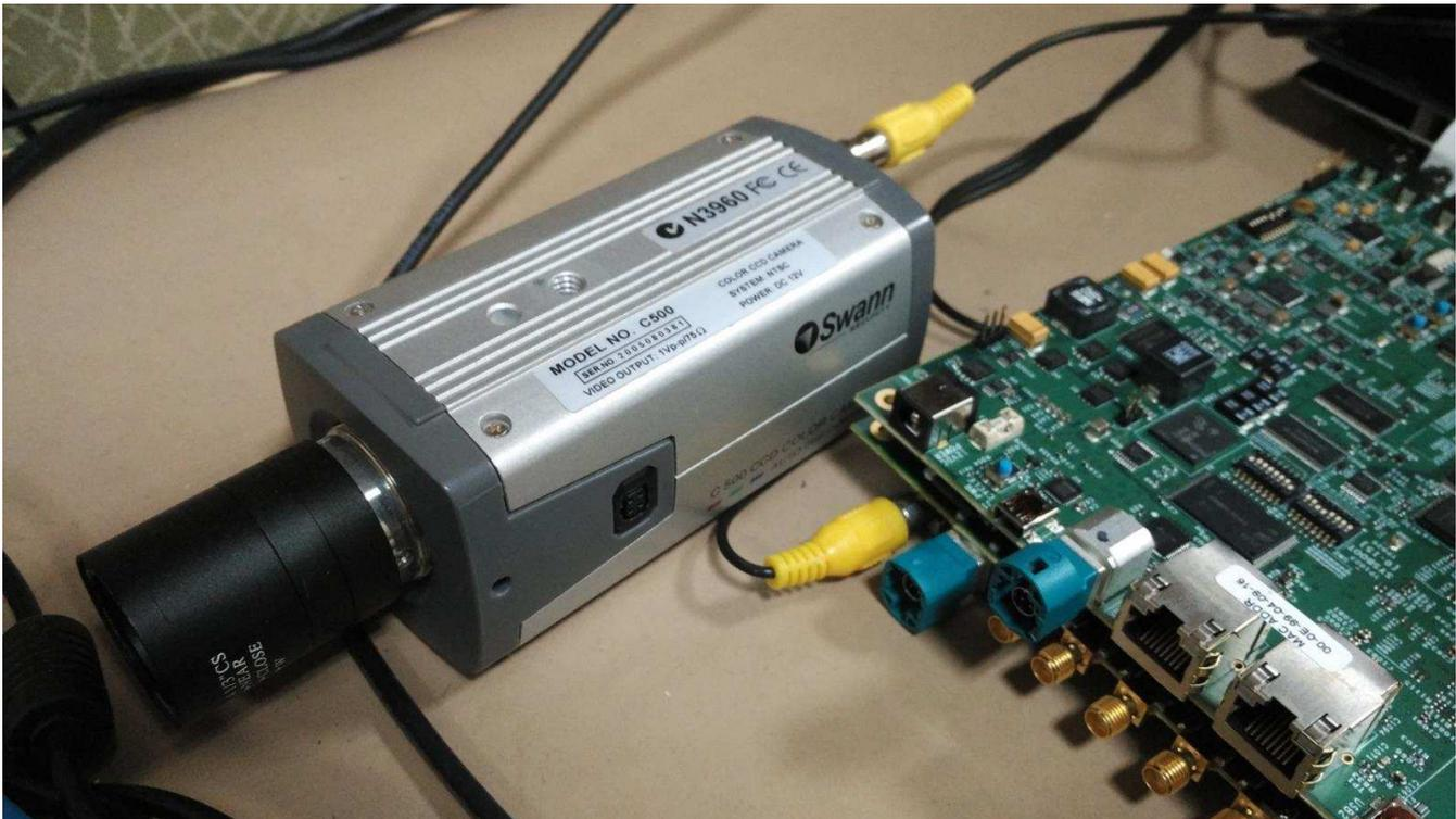
**Figure 3. analog camera via TVP5158**
