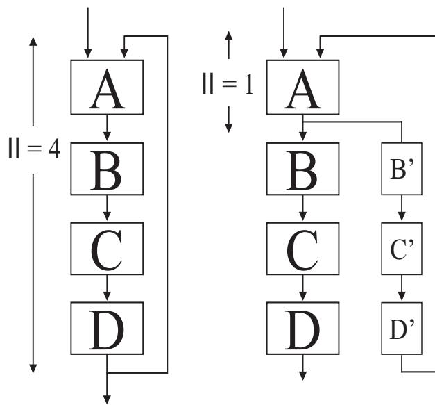
Figure 4 shows another solution to solve this dependence path and that is to copy a value and forward it as shown in the right side of the figure.
