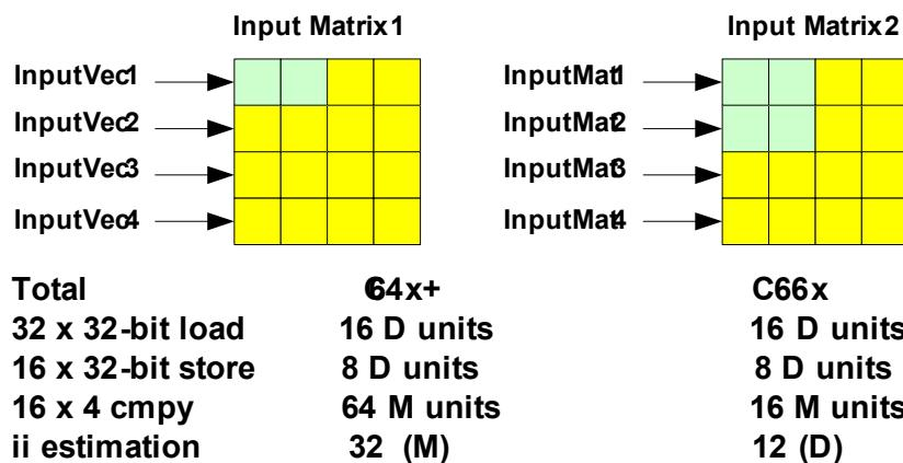
In this code, the C66x instructions CMATMPYR1 and DSADD2 are used. One ( $4 \times 4$ ) by ( $4 \times 4$ ) matrix multiplication is calculated per iteration.
