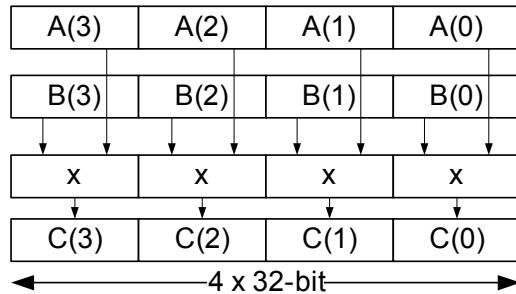
**SIMD Support**—Improved vector processing capability (each instruction can process multiple data in parallel) combined with the natural instruction level parallelism of C6000 architecture (e.g execution of up to 8 instructions per cycle) results in a very high level of parallelism that can be exploited by DSP programmers through the use of TI's optimized C/C++ compiler.
