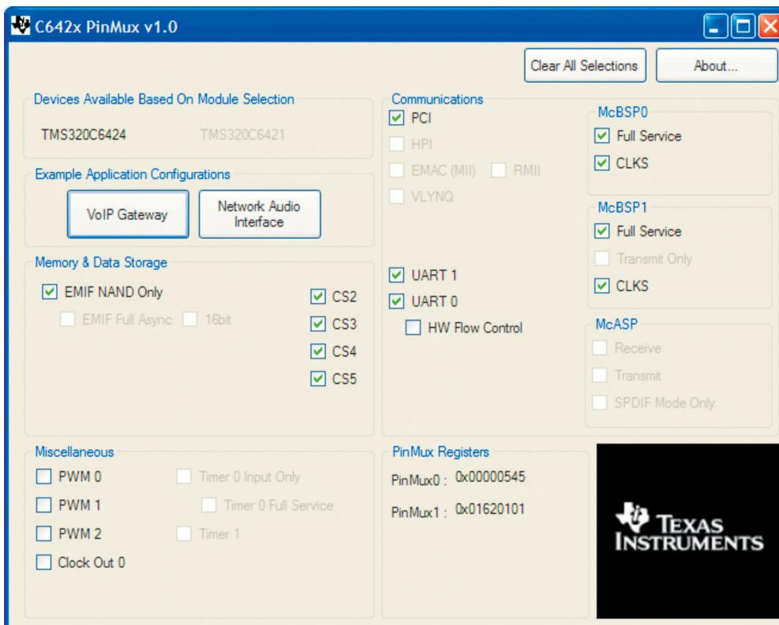
Figure 1. VoIP Gateway Configuration
