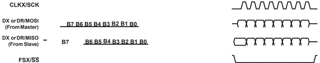
**Figure 2. SPI Transfer With CLKSTP = 11 and CLKXP = 0**
