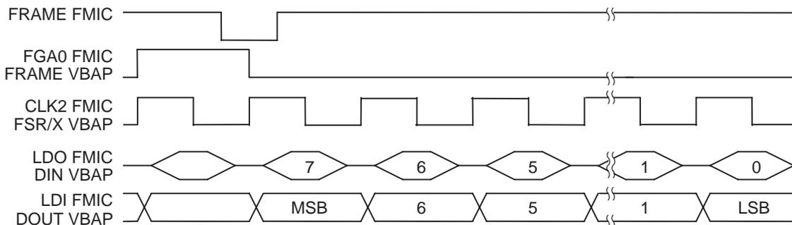
**Figure 3. VBAP and FMIC 2-MHz Mode Serial Timing**
