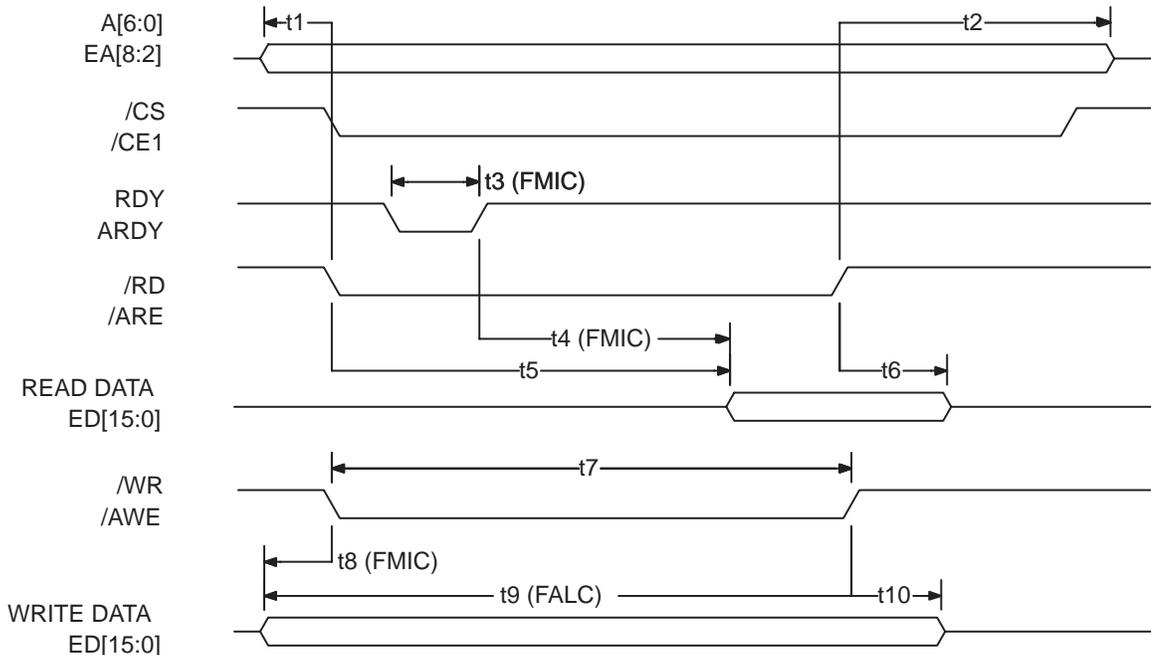
Figure 2. Combined Parallel Interface Timing
