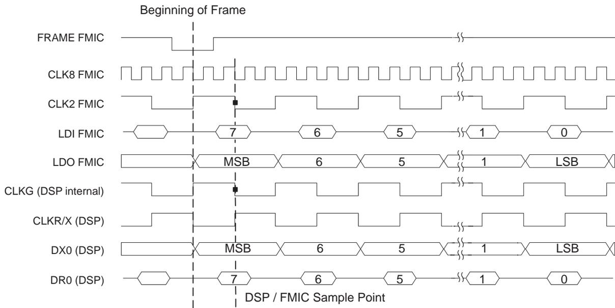
**Figure 4. DSP and FMIC 2-MHz Mode Serial Timing, With 8-MHz Clock**
