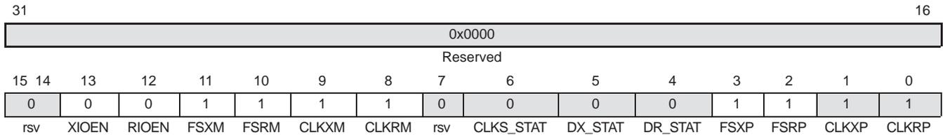
**Figure 5. Pin Control Register (PCR)**
