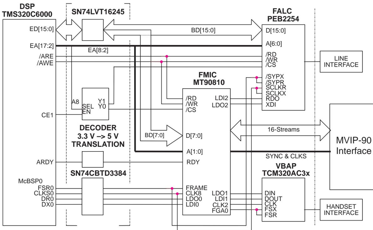
Figure 1. TMS320C6000 Interface to the FMIC, FALC, and VBAP
