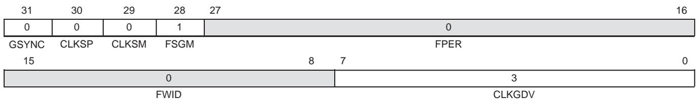
**Figure 6. Sample Rate Generator Register (SRGR)**
