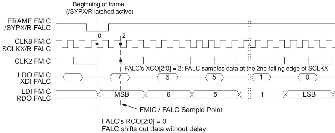
**Figure 7. FALC and FMIC 2-MHz Mode Serial Timing, With 8-MHz Clock**
