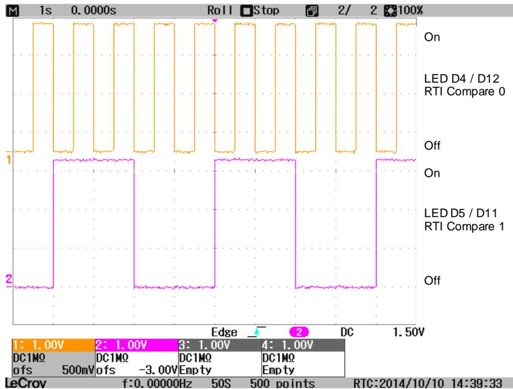
Figure 4. Oscilloscope Shot
