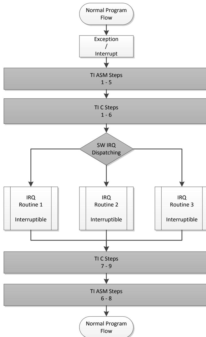
Figure 1. Program Flow With Common IRQ Handler
