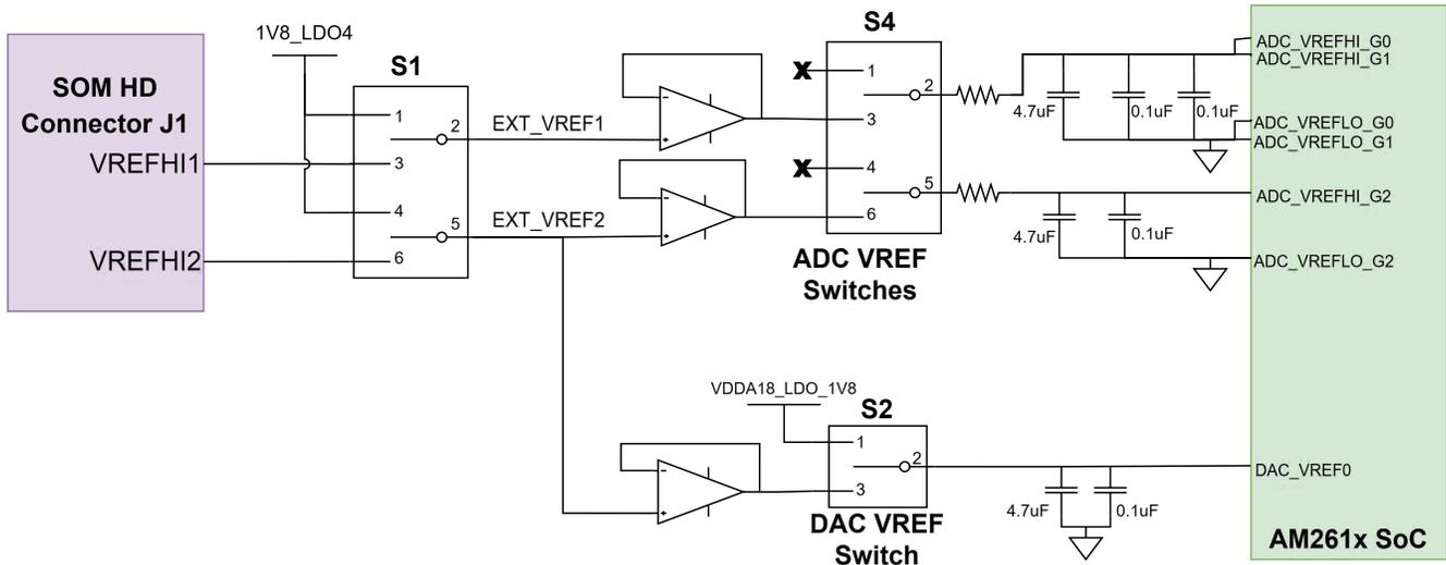
Figure 2-23. ADC Switch Routing
