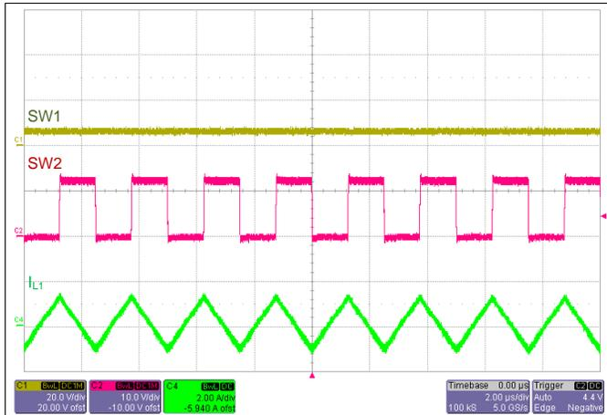
Figure 13. SW1, SW2,  $I_L$  Waveforms:  $V_{IN} = 6\text{ V}$ ,  $V_{OUT} = 12\text{ V}$ ,  $I_{OUT} = 0\text{ A}$
