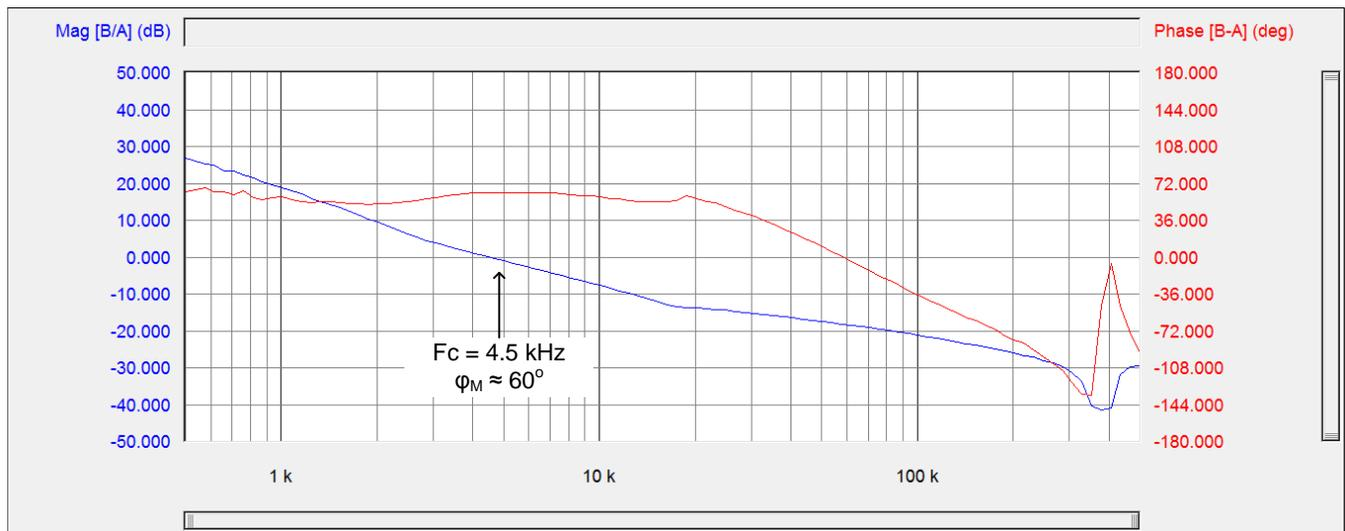
Figure 10. Bode Plot for  $V_{in} = 6V$ ,  $I_{out} = 3A$
