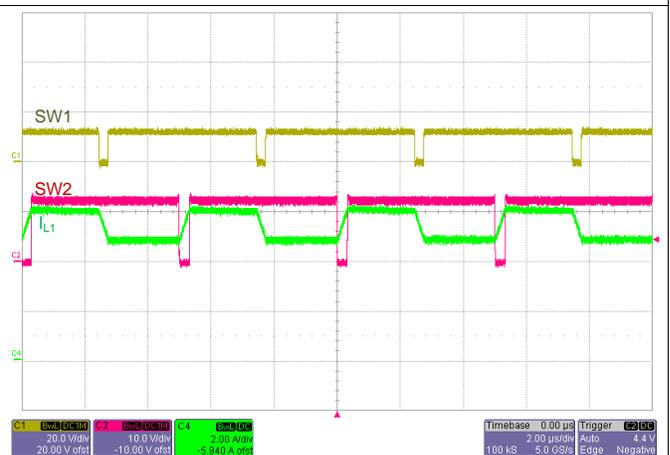
Figure 16. SW1, SW2,  $I_L$  Waveforms:  $V_{IN} = 12\text{ V}$ ,  $V_{OUT} = 12\text{ V}$ ,  $I_{OUT} = 5\text{ A}$
