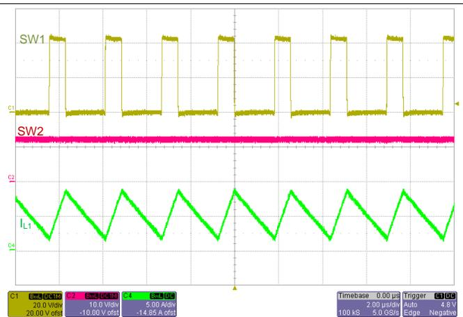
Figure 24. SW1, SW2,  $I_L$  Waveforms:  $V_{IN} = 42\text{ V}$ ,  $V_{OUT} = 12\text{ V}$ ,  $I_{OUT} = 5\text{ A}$
