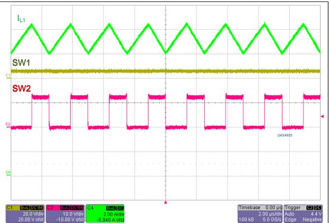
Figure 14. SW1, SW2,  $I_L$  Waveforms:  $V_{IN} = 6\text{ V}$ ,  $V_{OUT} = 12\text{ V}$ ,  $I_{OUT} = 5\text{ A}$
