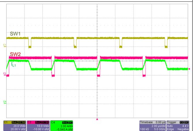
Figure 18. SW1, SW2,  $I_L$  Waveforms:  $V_{IN} = 16\text{ V}$ ,  $V_{OUT} = 12\text{ V}$ ,  $I_{OUT} = 5\text{ A}$
