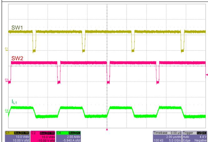
Figure 15. SW1, SW2,  $I_L$  Waveforms:  $V_{IN} = 12\text{ V}$ ,  $V_{OUT} = 12\text{ V}$ ,  $I_{OUT} = 0\text{ A}$
