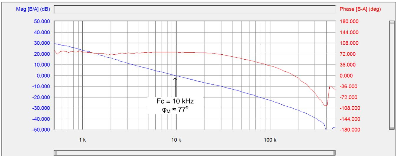
Figure 12. Bode Plot for  $V_{IN} = 24V$ ,  $I_{OUT} = 3A$
