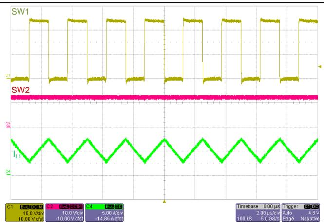
Figure 22. SW1, SW2,  $I_L$  Waveforms:  $V_{IN} = 24\text{ V}$ ,  $V_{OUT} = 12\text{ V}$ ,  $I_{OUT} = 5\text{ A}$
