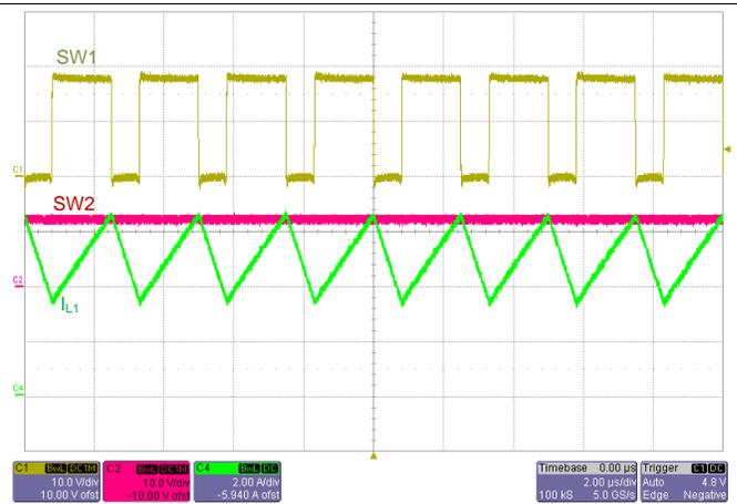
Figure 20. SW1, SW2,  $I_L$  Waveforms:  $V_{IN} = 18\text{ V}$ ,  $V_{OUT} = 12\text{ V}$ ,  $I_{OUT} = 5\text{ A}$
