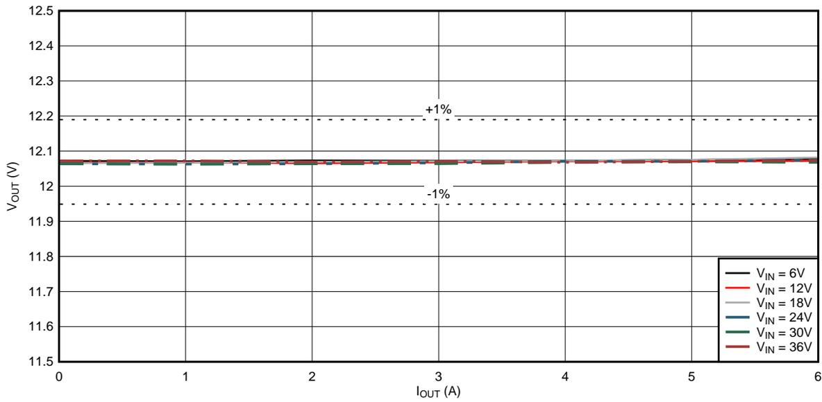
Figure 9. Line and Load Regulation
