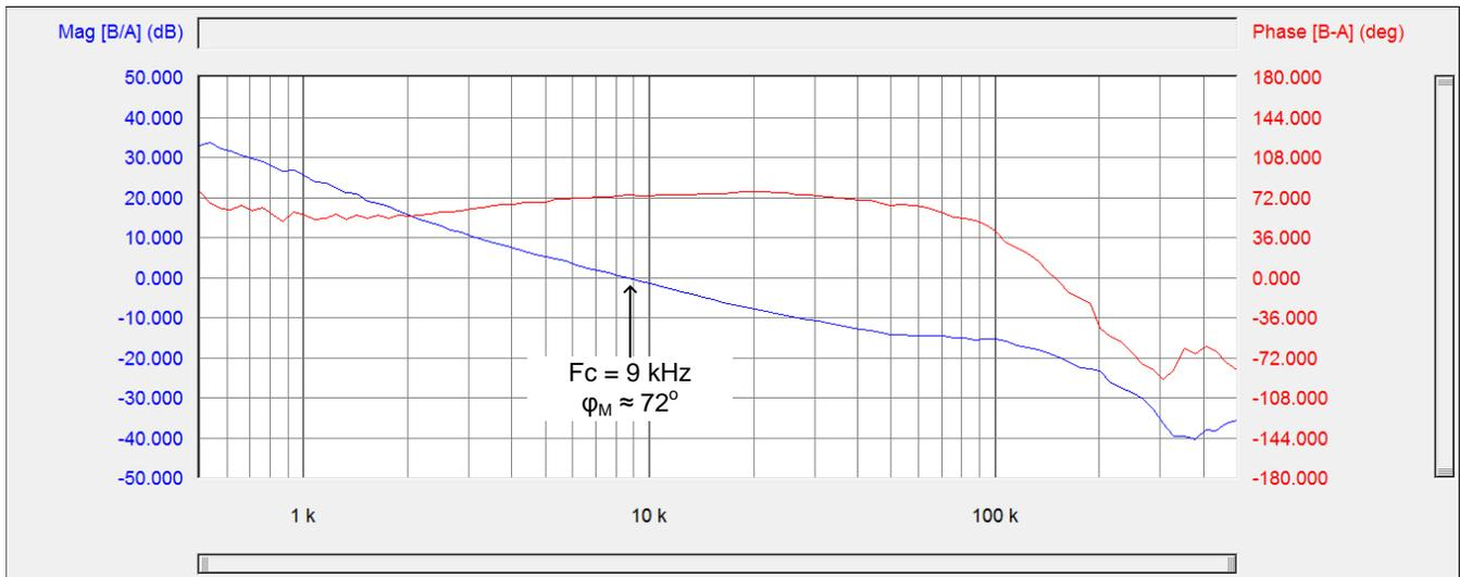
Figure 11. Bode Plot for  $V_{IN} = 12V$ ,  $I_{OUT} = 3A$
