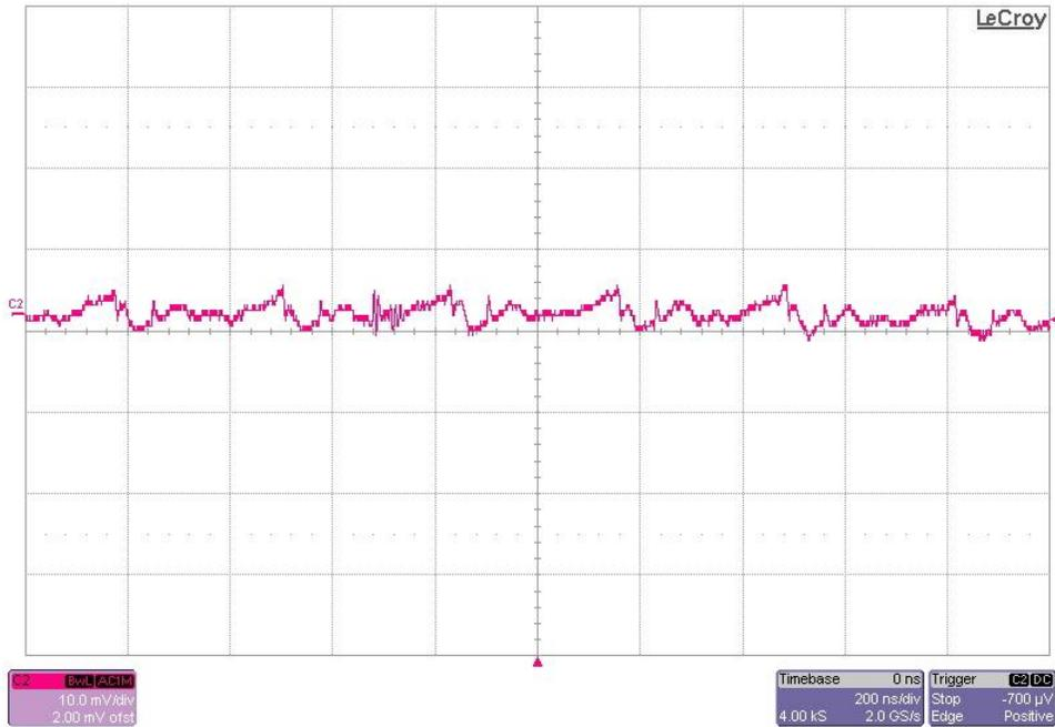
The 1.1V output ripple voltage is shown in the figure below. The image was taken with the output loaded to 2A. The input voltage is set to 5V. (10mV/DIV, 200nS/DIV)
