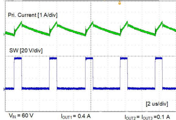
Figure 5-4. Steady State When  $V_{IN}=60\text{ V}$ ,  $I_{OUT1}=0.4\text{ A}$ ,  $I_{OUT2}=I_{OUT3}=0.1\text{ A}$
