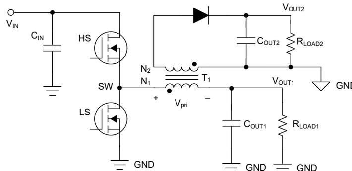
**Figure 2-1. General Fly-Buck Converter Circuit**
