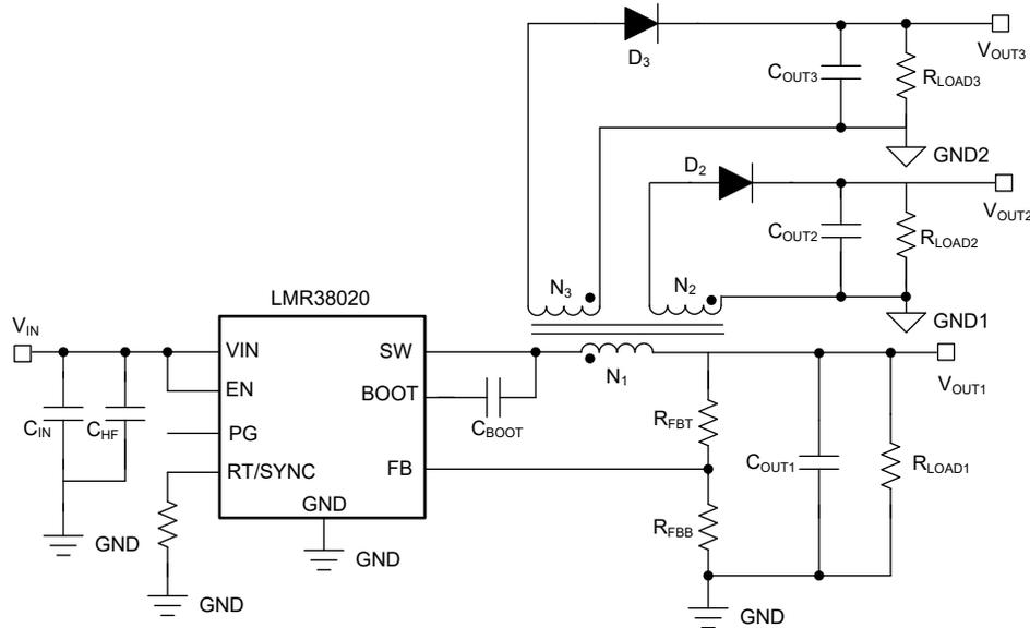
Figure 4-1. Fly-Buck Converter With LMR38020
