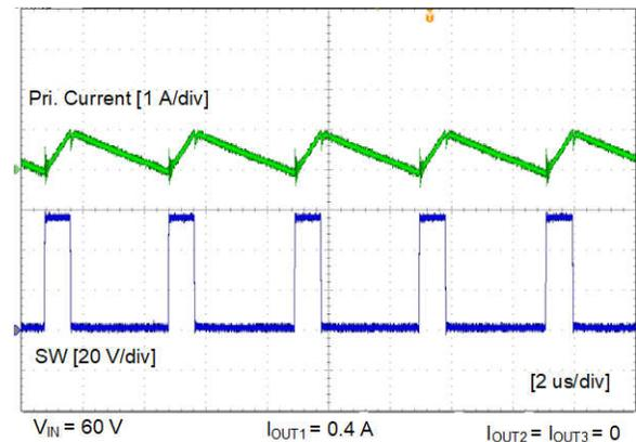
Figure 5-6. Steady State When  $V_{IN}=60\text{ V}$ ,  $I_{OUT1}=0.4\text{ A}$ ,  $I_{OUT2}=I_{OUT3}=0\text{ A}$
