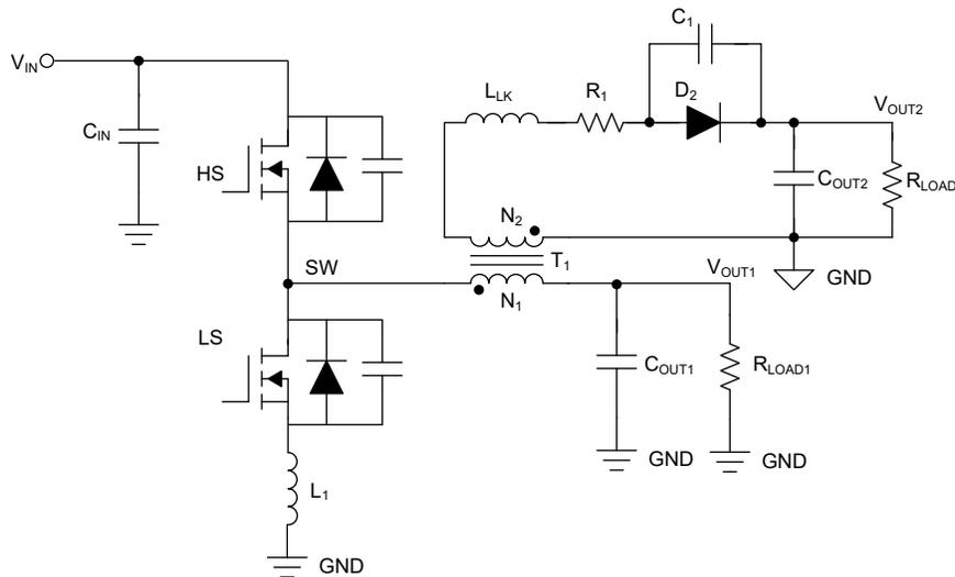
**Figure 3-2. Fly-Buck Converter Circuit Considering Parasitic**
