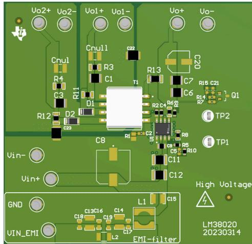
Figure 5-2. LMR38020 Fly-Buck Demo Board
