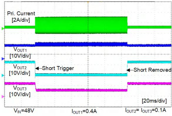
Figure 5-14. Short Circuit On Secondary Output
