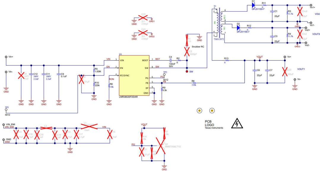
Figure 5-1. LMR38020 Fly-Buck Converter Schematic
