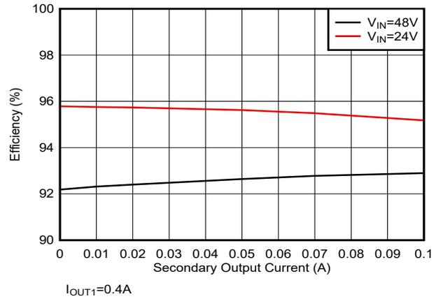
Figure 5-10. Efficiency :  $I_{OUT1}=0.4 A$
