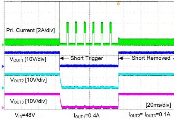
Figure 5-13. Short Circuit On Primary Output
