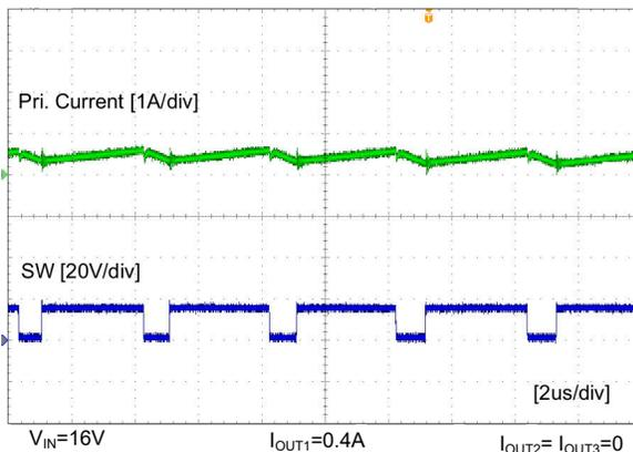
Figure 5-5. Steady State When  $V_{IN}=16\text{ V}$ ,  $I_{OUT1}=0.4\text{ A}$ ,  $I_{OUT2}=I_{OUT3}=0\text{ A}$
