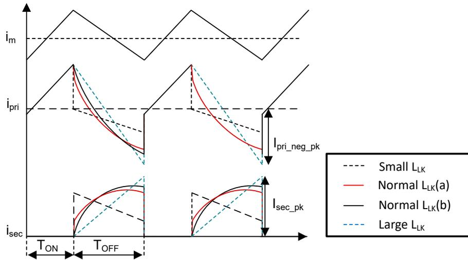
Figure 3-3. Current Waveforms Affected by Leakage Inductance
