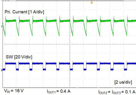
Figure 5-3. Steady State When  $V_{IN}=16\text{ V}$ ,  $I_{OUT1}=0.4\text{ A}$ ,  $I_{OUT2}=I_{OUT3}=0.1\text{ A}$
