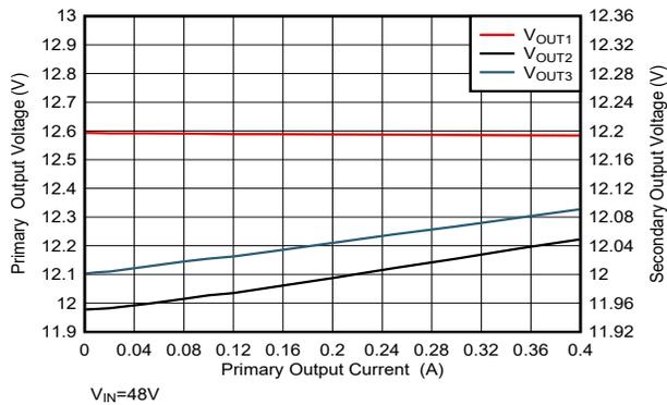
Figure 5-11. Load Regulation vs Primary Output Current
