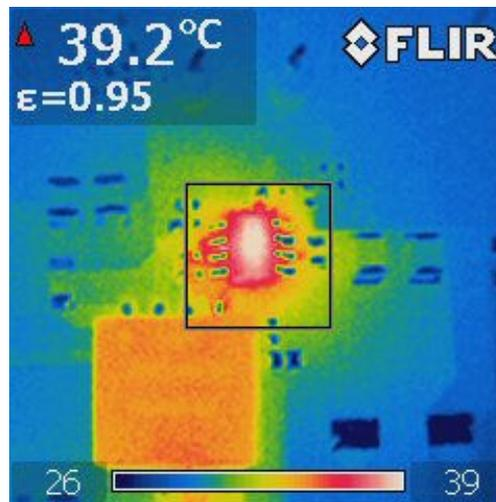
Figure 5-15. Thermal Performance When  $V_{IN}=48\text{ V}$ , Full Load
