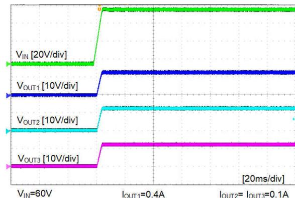
Figure 5-8. Start Up When  $V_{IN}=60\text{ V}$ , Full Load
