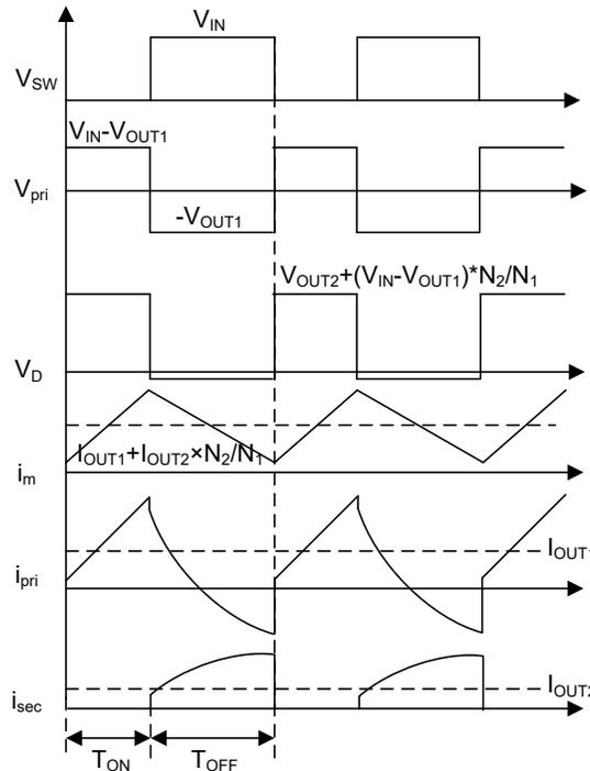
Figure 3-1. Fly-Buck™ Steady State Operation Waveforms
