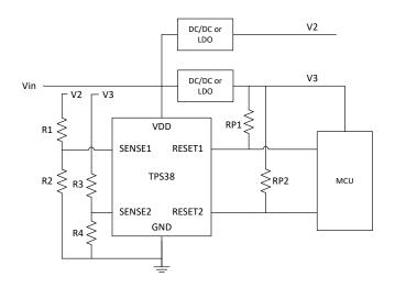
Device shown: TPS38A010122DSKRQ1 adjustable threshold variant
