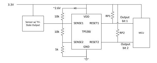
Device shown: TPS38J010155DSKRQ1 adjustable threshold variant
