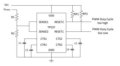
Device shown: TPS37A010122DSKR adjustable threshold variant
