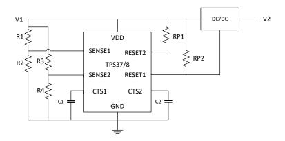
**Device shown:** TPS37A010122DSKR adjustable threshold variant or TPS38A010122DSKRQ1 adjustable threshold variant
