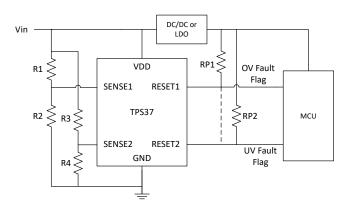
**Device shown:** TPS37A010122DSKR adjustable threshold variant **Additional resources:** TPS37 data sheet section 10.1
