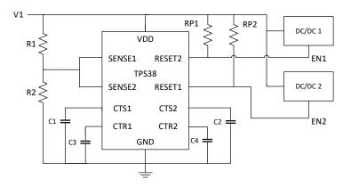
**Device shown:** TPS38A010122DSKRQ1 adjustable threshold variant **Additional resources:** TPS38 data sheet section 8.3.4 TPS38 online design calculator
