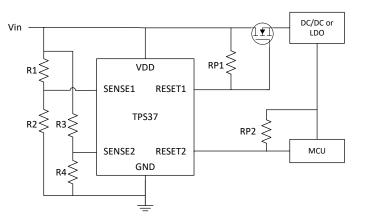
Device shown: TPS37A010122DSKR adjustable threshold variant
