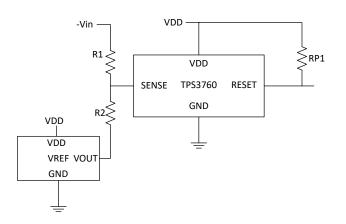
Device shown: TPS3760A012DYYR adjustable threshold variant
