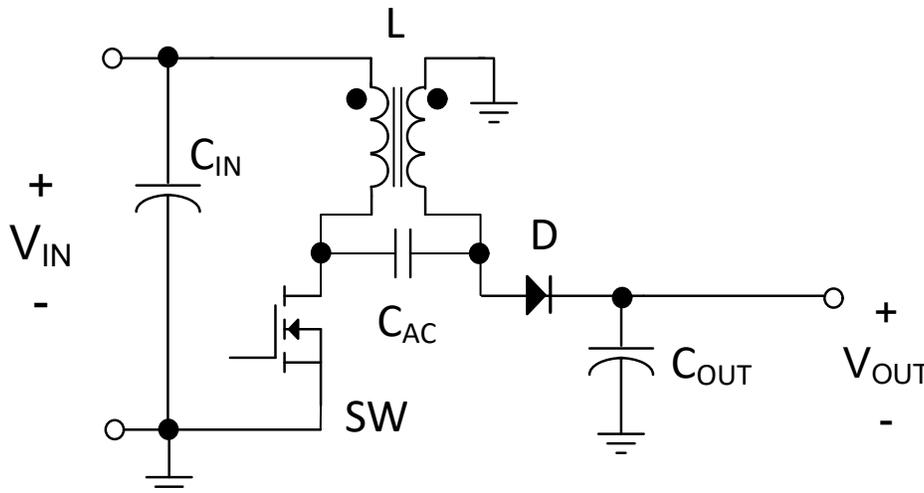
**Figure 1-1. Coupled Inductor SEPIC Power Stage**
