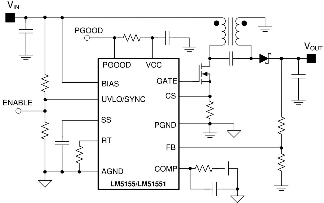
Figure 4-1. Application Circuit
