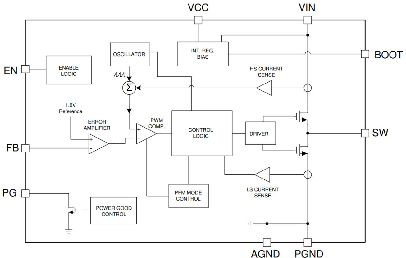
**Figure 1-1. Functional Block Diagram: LM60430, LM60440**
