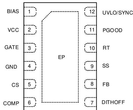
**Figure 5-1. Pin Diagram**
