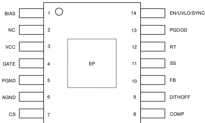
**Figure 6-1. Pin Diagram LM5156H, LM5156H-Q1, LM51561H, LM51561H-Q1**
