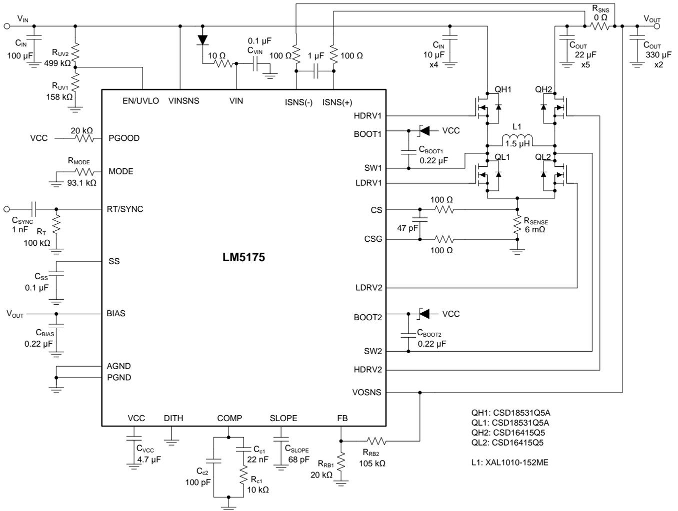
Figure 3. Complete Application Schematic for an Automotive Design For Cold-crank
