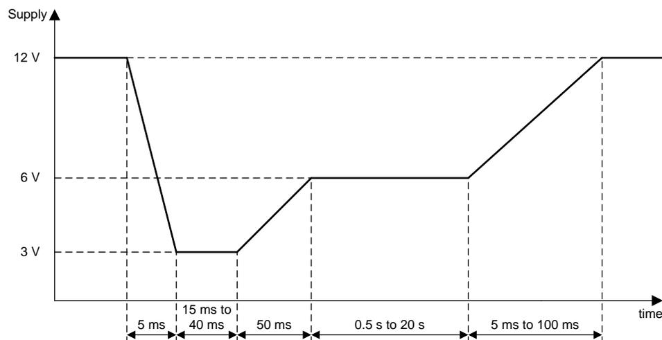
**Figure 1. A Representative Startup (Cold-crank) Test Profile for Car Supply with 12-V Battery**
