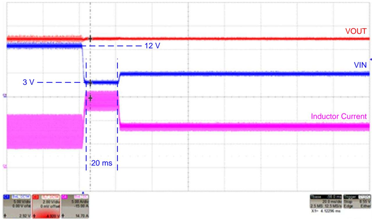
Figure 2. VOUT Regulated to 5 V as the Input Supply Voltage Drops Below 3 V for 20ms (Load=7.5 A)
