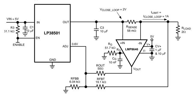
Figure 1. Resistive Load Application with LP38501 Regulator
