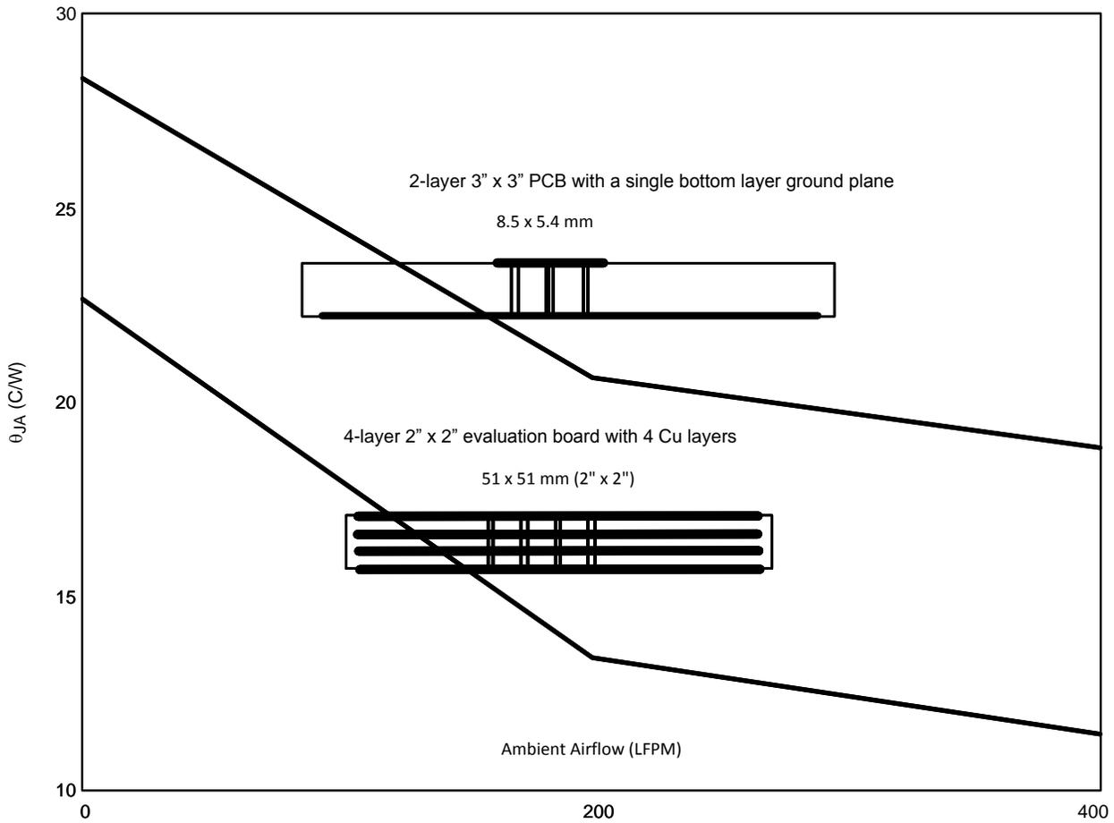
Figure 5. Effect of Airflow for Two PCBs
