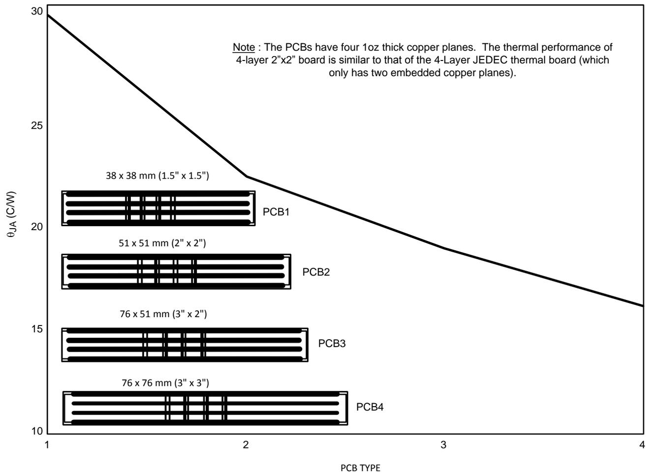
Figure 3. Effect of PCB Size of 4-Layer PCB
