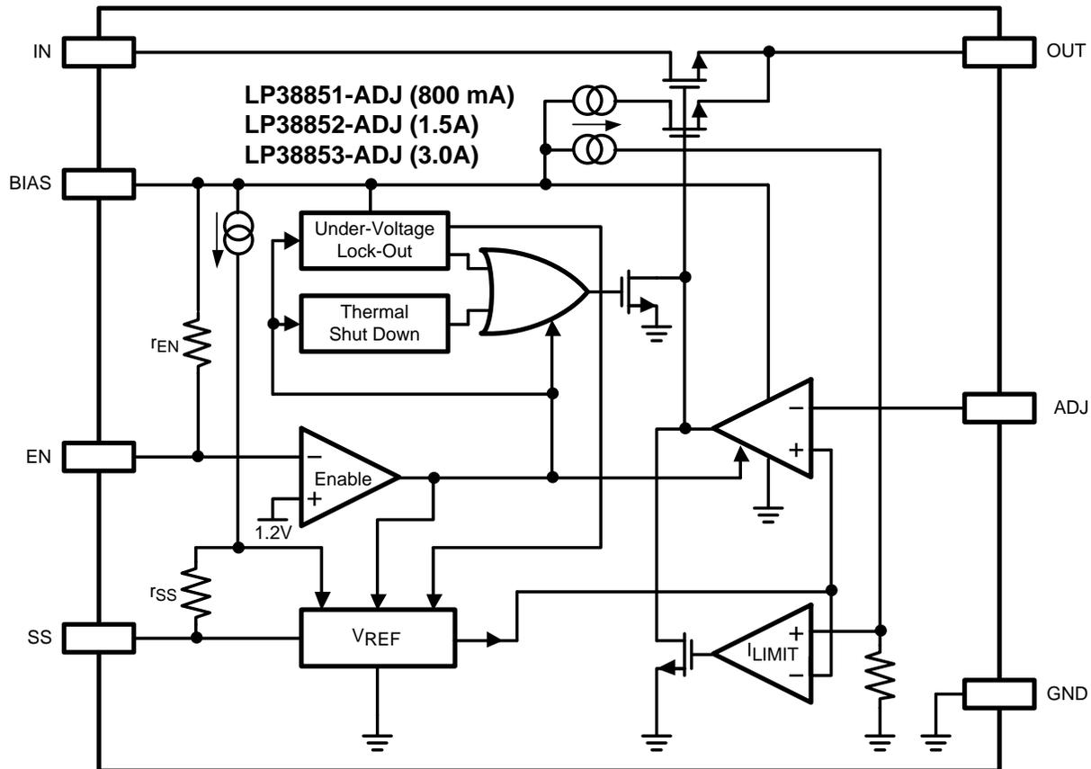
**Figure 1. LP38851/52/53-ADJ Block Diagram**
