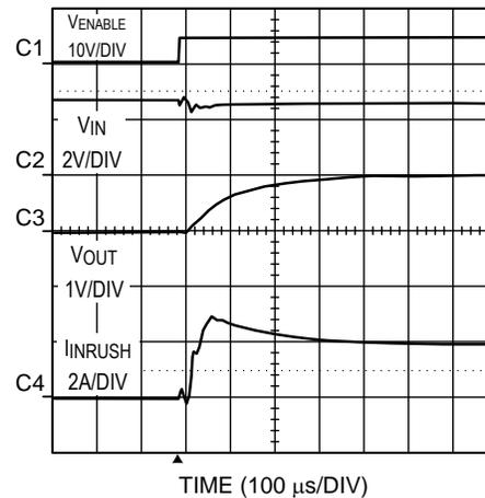
**Figure 4. Startup In-Rush Current With Soft-start,  $C_{OUT} = 330\ \mu\text{F}$**
