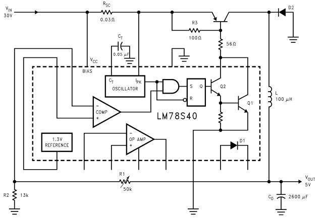
Figure 13. Modified Step-Down Regulator with 5A, 5V Output
