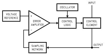
Figure 2. Regulator System Block Diagrams
