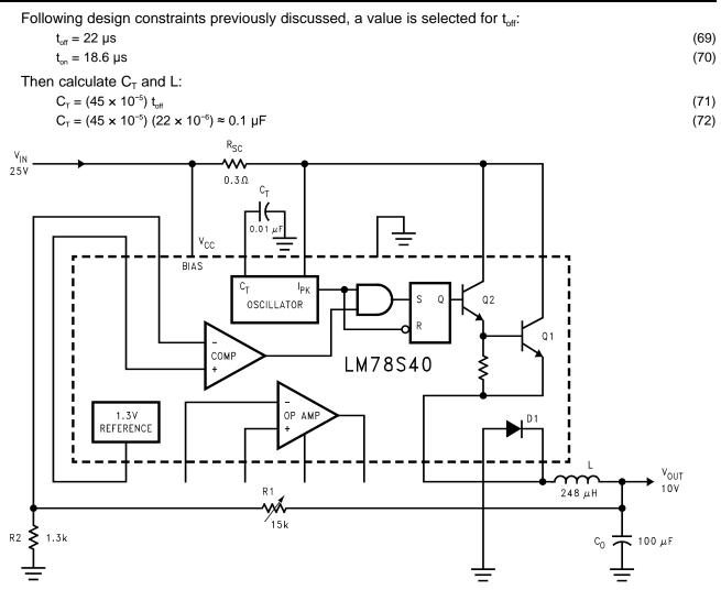
Figure 12. Step-Down Voltage Regulator
