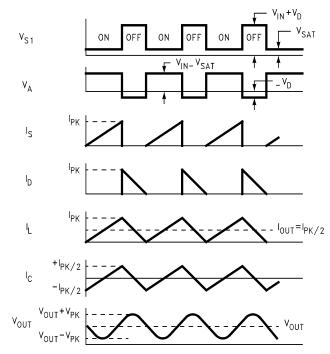
Figure 7. Waveforms for Step-Down Mode
