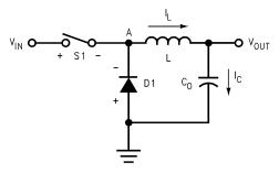
Figure 3. Basic Operating Mode: Step-Down Configuration
