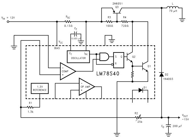
Figure 14. Inverting Regulator
