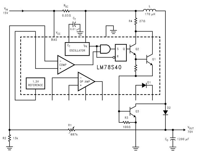
Figure 11. Switching Regulator with 15V Input, 70V Output
