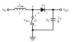
Figure 4. Basic Operating Mode: Step-Up Configuration
