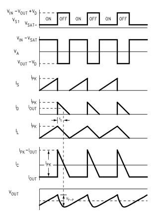
Figure 9. Voltage Inverter Waveforms
