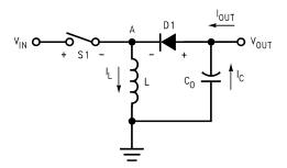
Figure 5. Basic Operating Mode: Inverting Configuration
