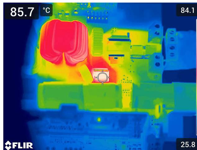
Figure 4-31. Relay Bypass Switch Thermal Image
