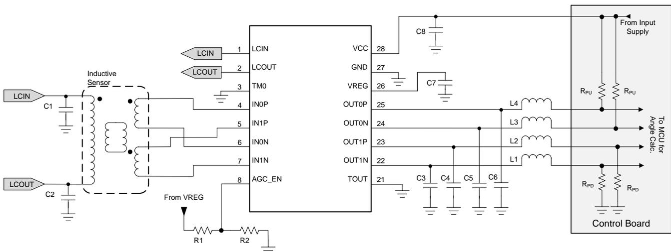
**Figure 1. Typical Application Diagram**
