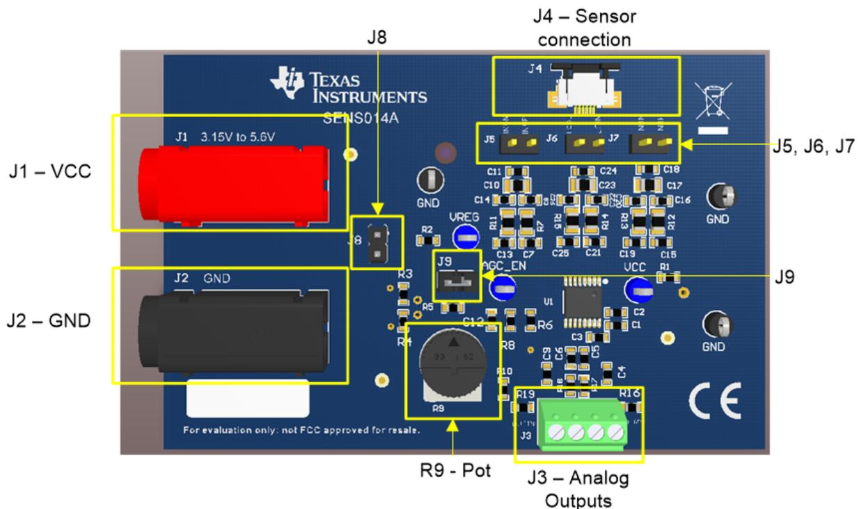
**Figure 2. Connector and Feature Locations**
