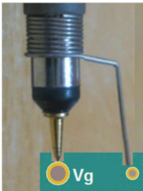
Figure 9-2. Recommended Use for Ground Spring Clip Test Points
