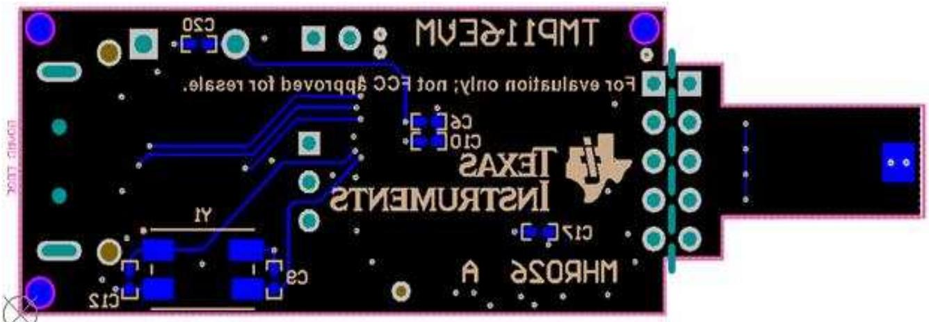
Figure 26. Bottom Assembly Layer
