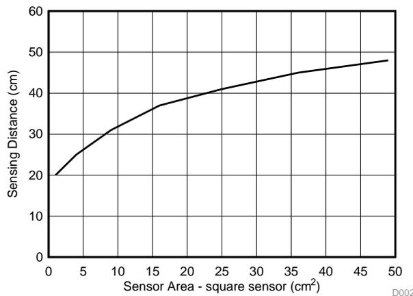
**Figure 4. Sensor Size Area Versus Sensing Distance**
