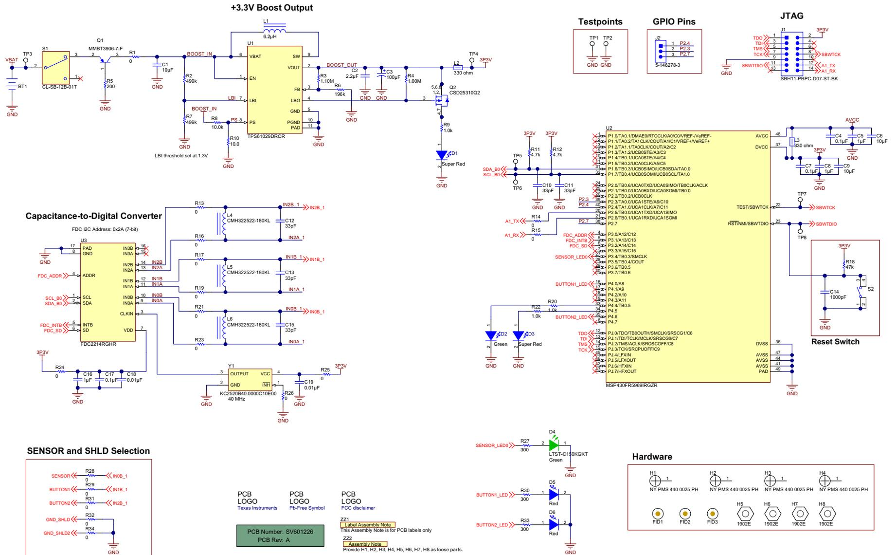
Figure 15. Schematic
