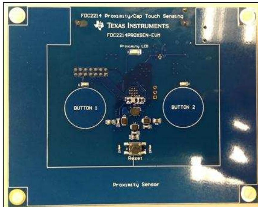
**Figure 1. FDC2214 Proximity and Capacitor Touch Sensing EVM**
