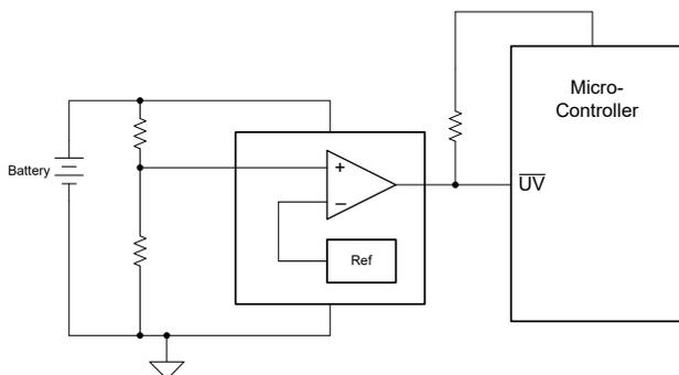
**Figure 7. Undervoltage Detection using an Integrated Reference Comparator**
