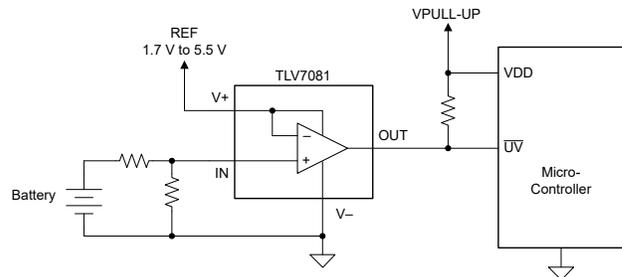
**Figure 5. Voltage Monitoring using the TLV7081**
