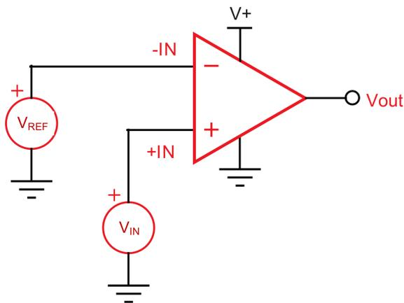
**Figure 1. Non-inverting Comparator Configuration**
