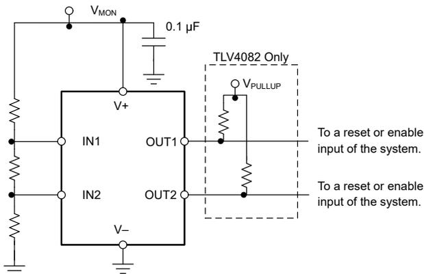
**Figure 9. Multi-Level Voltage Detection using TLV4062 and TLV4082**
