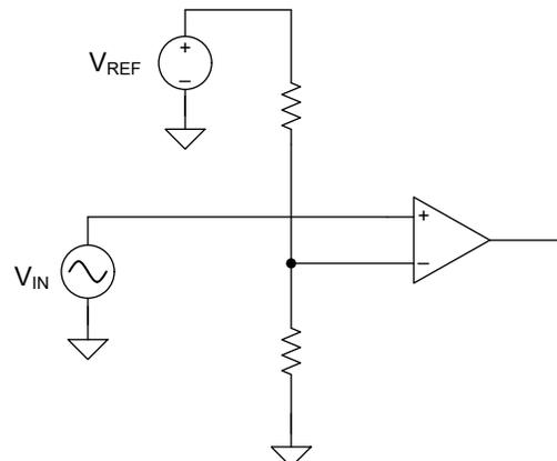
**Figure 2. Using Resistors to Create an External Reference**
