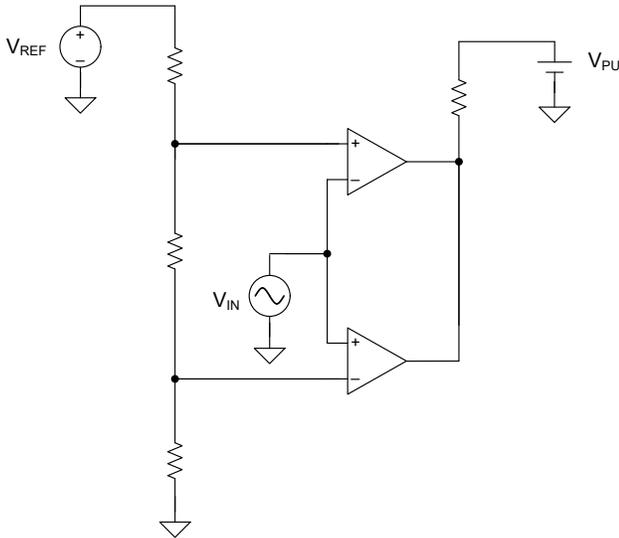
**Figure 3. Window Comparator Configuration**
