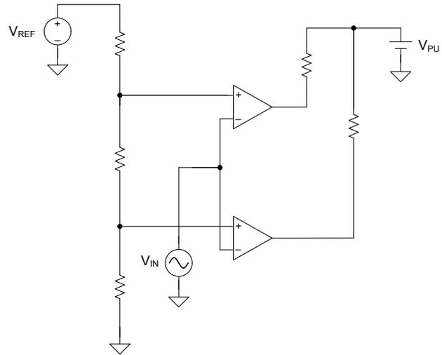
**Figure 4. Multi-stage Voltage Detection Circuit**
