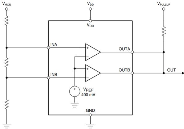
**Figure 8. Voltage Monitoring using Window Comparators TLV6700/6710**
