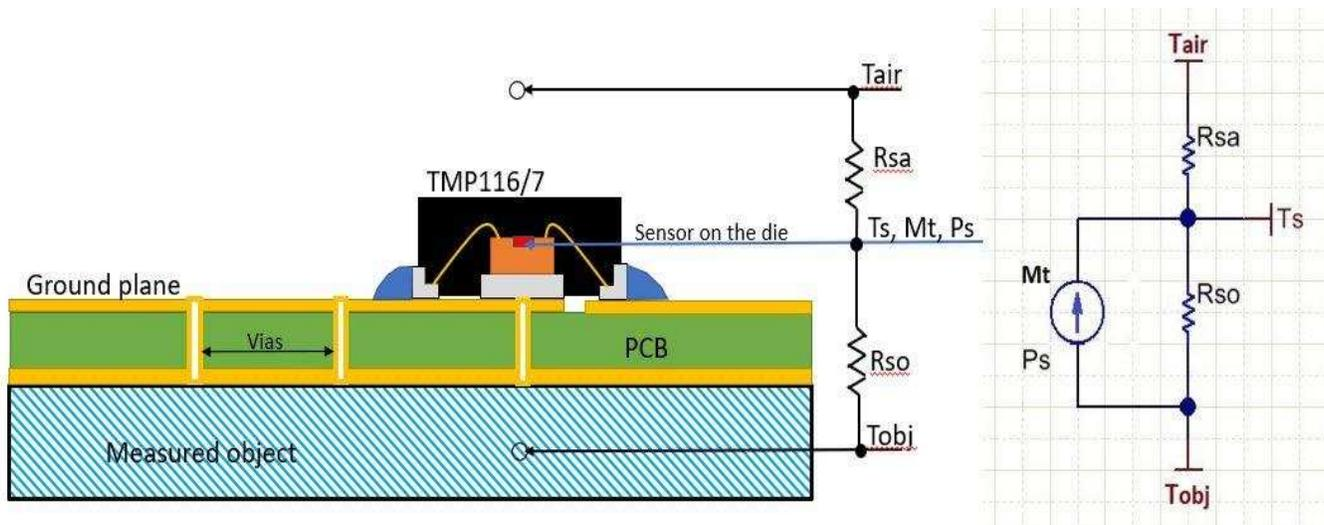
**Figure 1. Simplified Schematic of Temperature Flow During Solid Surface Measurement**
