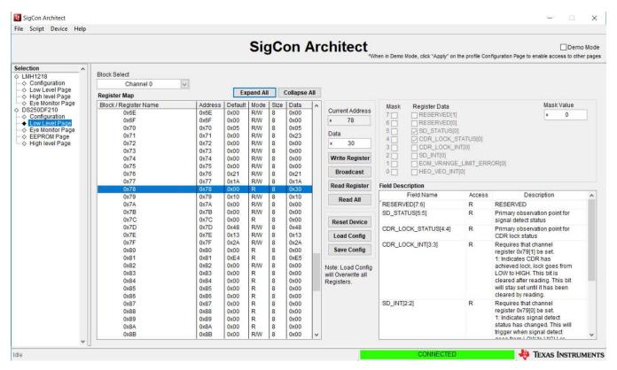
Figure 6. Low-Level Page Capture After Selecting Access to an Individual Register
