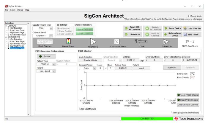
Figure 19. PRBS Tab, PRBS Checker Configuration
