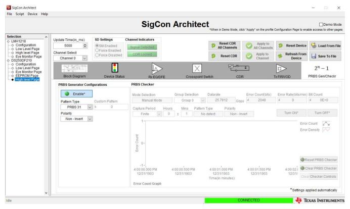
Figure 18. PRBS Tab, PRBS Generator Configuration
