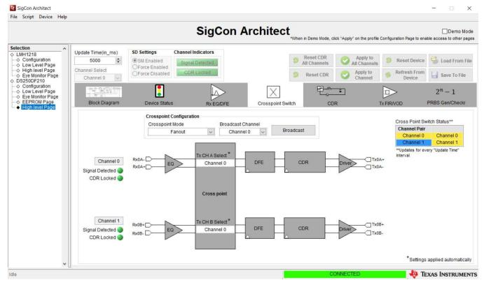
Figure 13. Cross-Point Tab, Fanout Mode Selected
