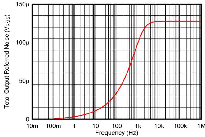
Figure 2-3. Integrated Noise of AFE
