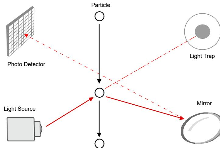
**Figure 1-1. Light Scattering Concept of Optical PM Instruments**
