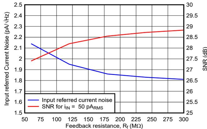
**Figure 3-1. SNR vs. Feedback Resistance**
