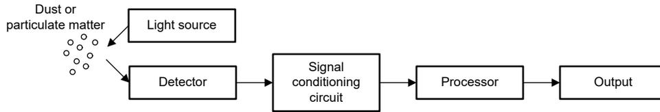
**Figure 1-2. Block Diagram PM Sensor**
