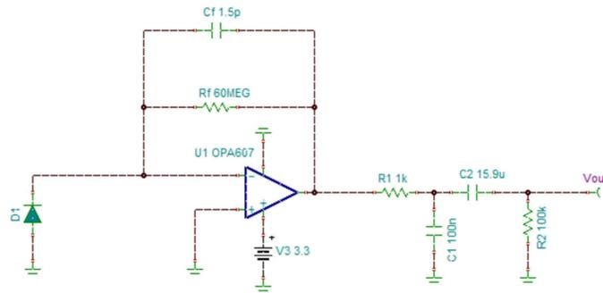
**Figure 2-1. Block Diagram of Analog Front End (AFE)**
