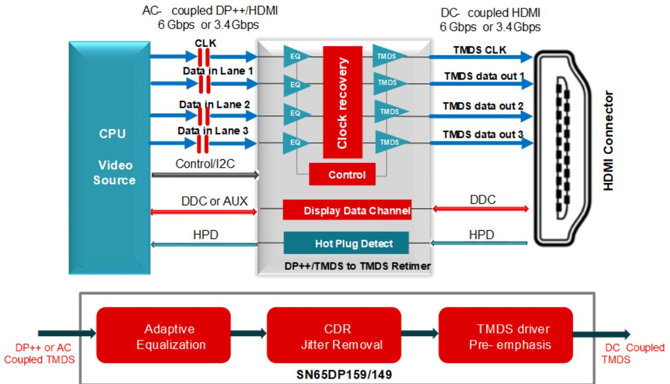
Figure 2-5. HDMI2.0 Retimer Example Using TI SN65DP159
