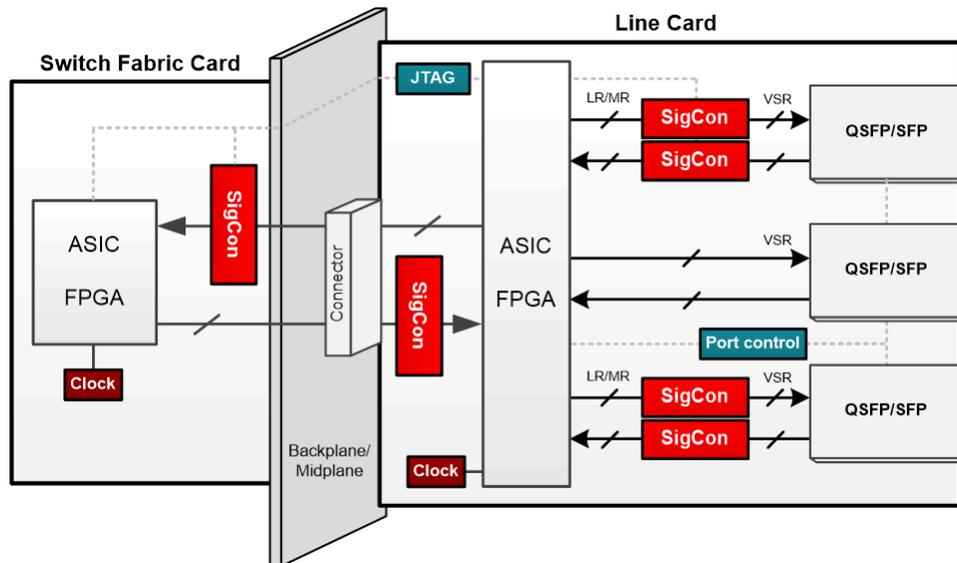
**Figure 2-7. 10GbE Communication Switch using Ethernet Retimer**
