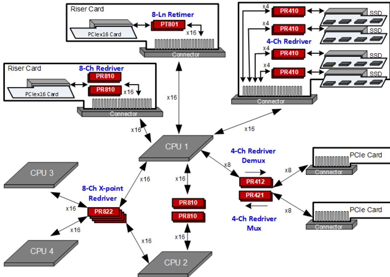
**Figure 2-6. PCIe 4.0 Signal Conditioner Functions Using TI Redriver and Retimers**
