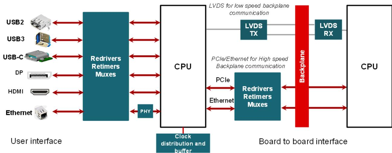
**Figure 2-2. High speed interfaces inside an industrial PC system**
