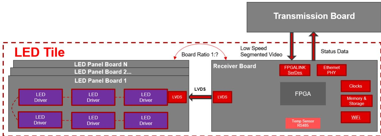
Figure 2-5. Receiver Board
