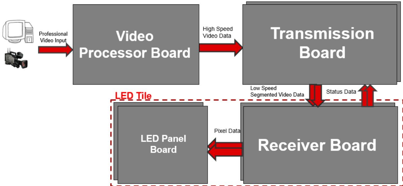
Figure 2-1. LED Wall Functional Block Diagram
