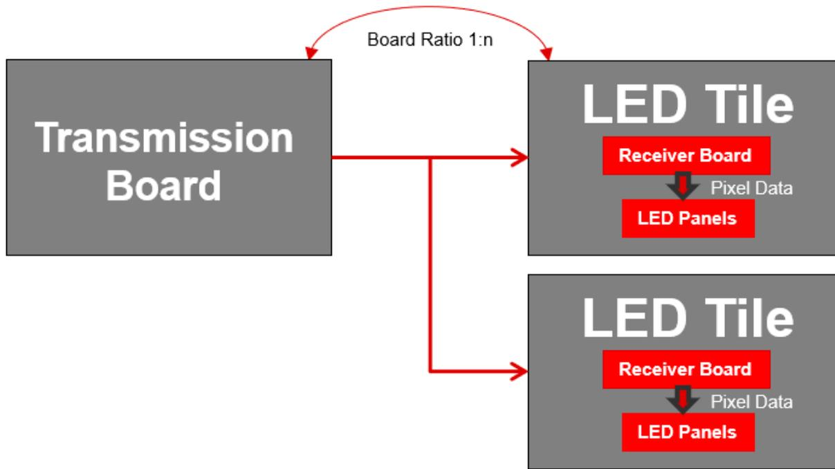
Figure 2-4. Daisy Chained Transmission Board
