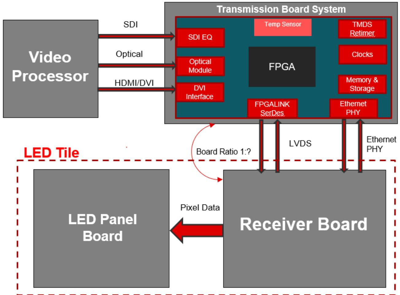
Figure 2-3. Transmission Board
