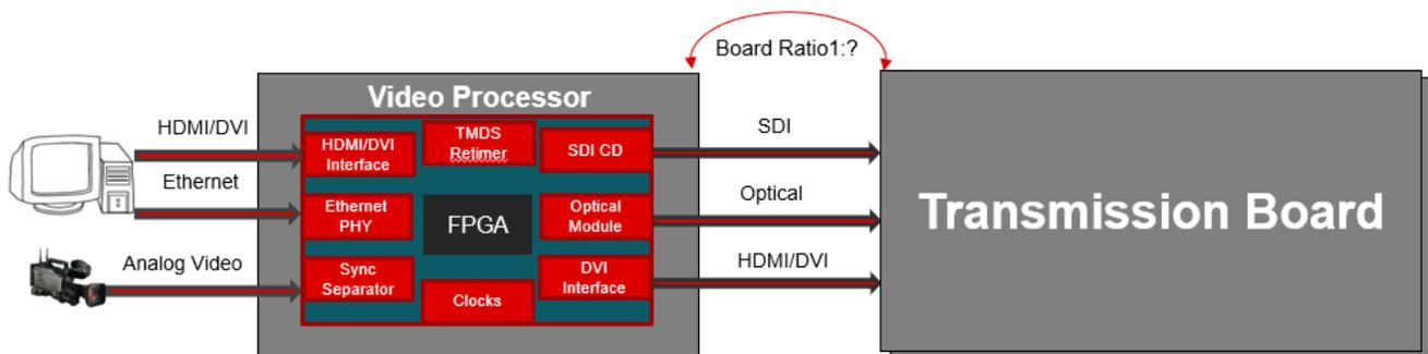
Figure 2-2. Processor Board
