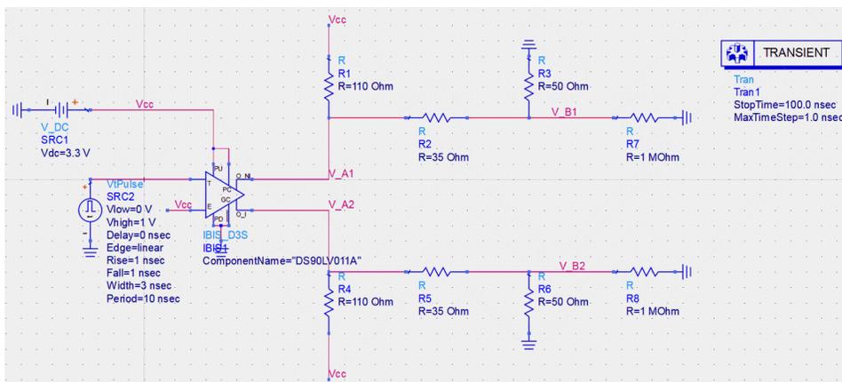
**Figure 3-2. Schematic for Receivers Without Internal Termination**
