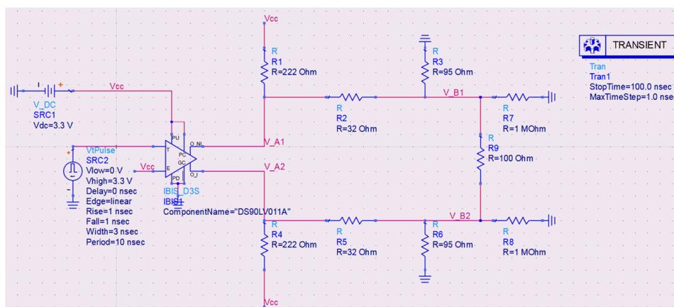
**Figure 4-2. Schematic for Receivers With Internal Termination**
