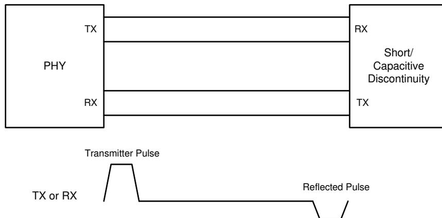
**Figure 2. Short Circuit Cable**
