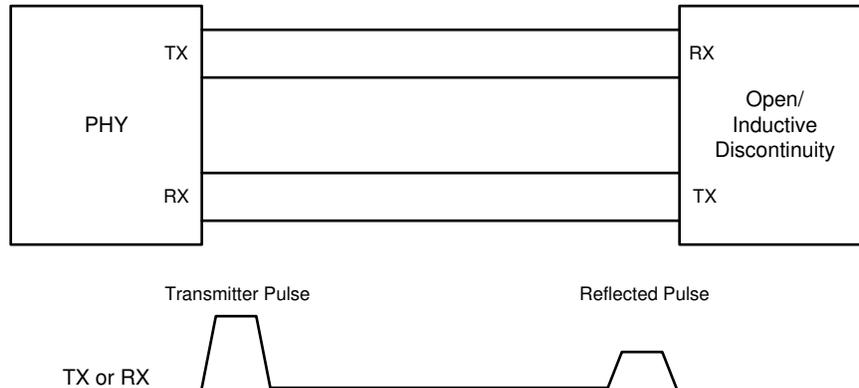
**Figure 1. Open Circuit Cable**
