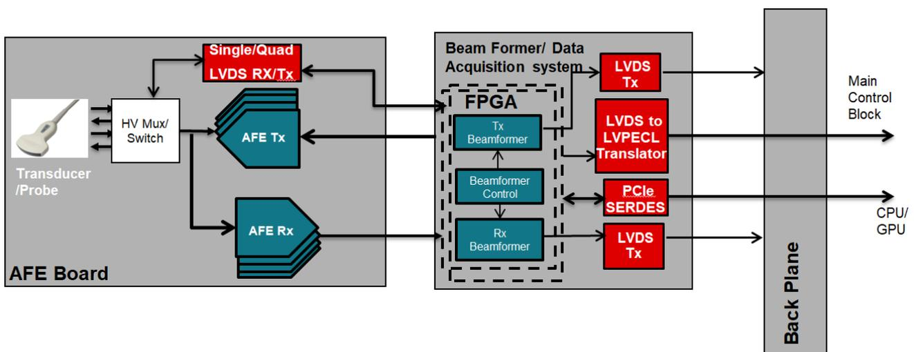
Figure 2. AFE Board and Beamformer Subsystem
