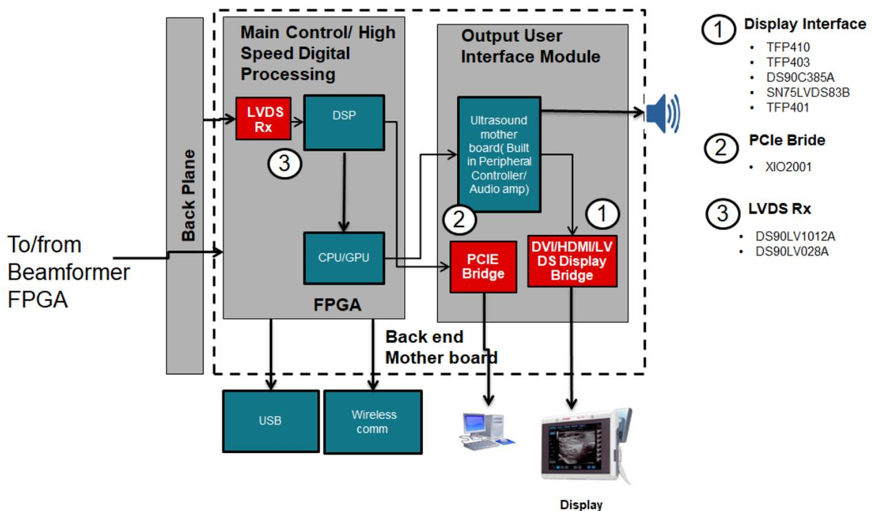
**Figure 4. DSP and User Interface Subsystem**
