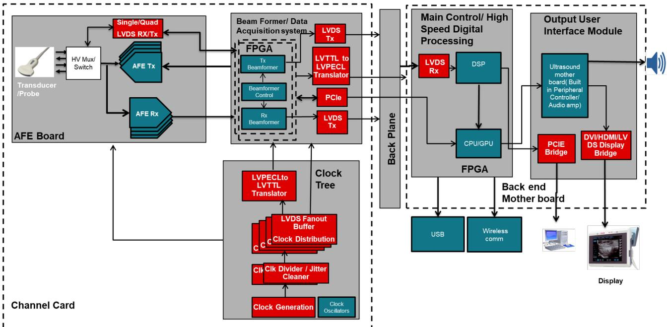
Figure 1. Ultrasound Scanner Simplified Block Diagram
