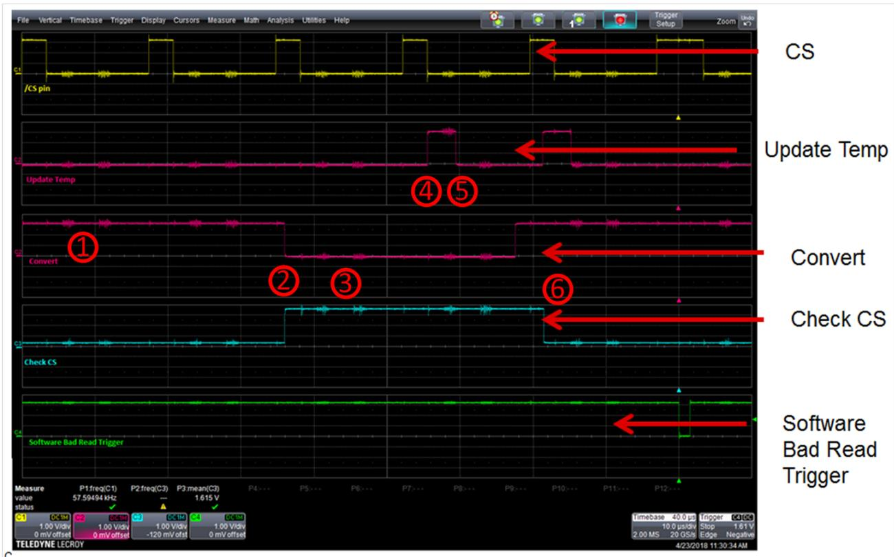
**Figure 3. Oscilloscope Capture of Erroneous Result Update**
