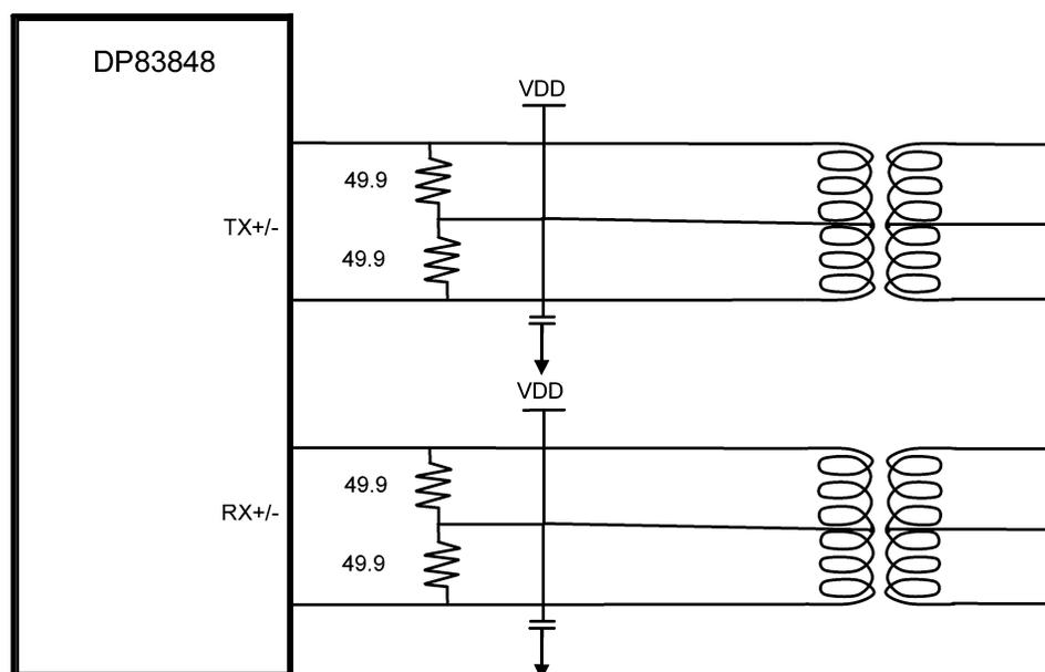
**Figure 2. DP83848C/I/YB PMD Connections (Termination and Biasing)**
