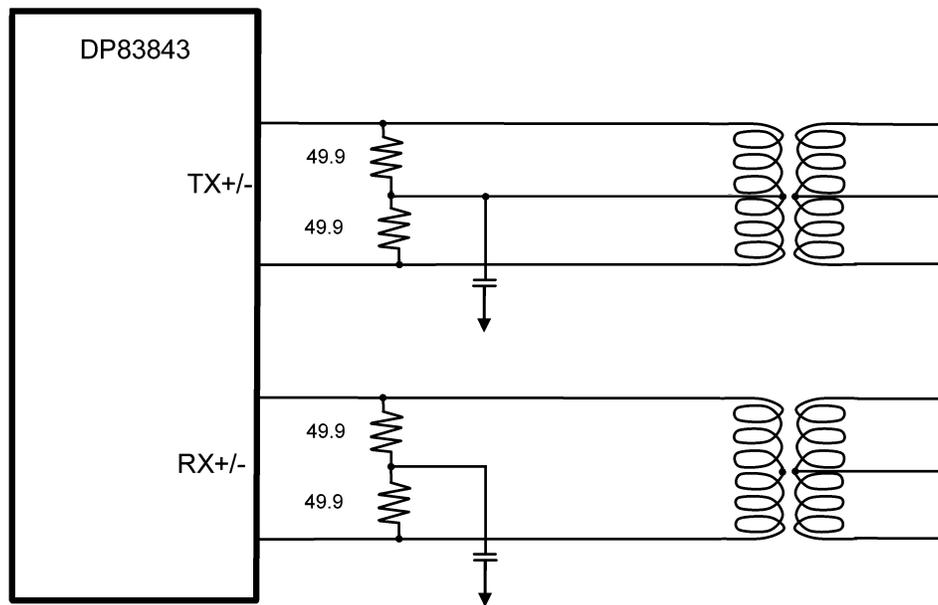
Figure 3. DP83843 PMD Connections (Termination and Biasing)
