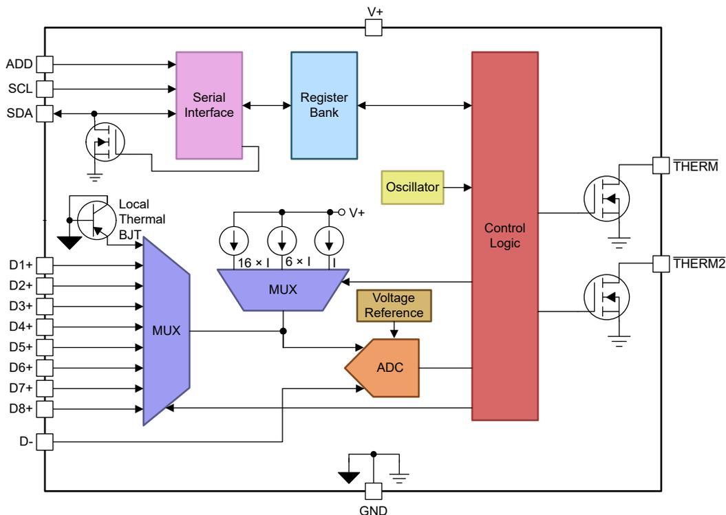
Figure 2-1. Functional Block Diagram of the TMP9R00-SP
