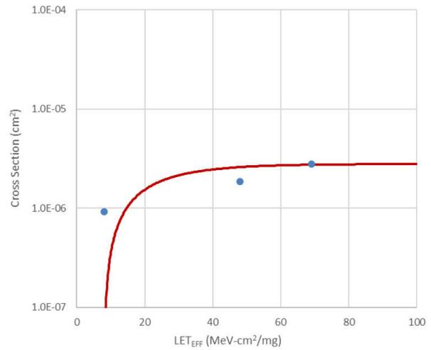
Figure 3-11. Weibull Plot: V+ 1.7 V - Local Channel
