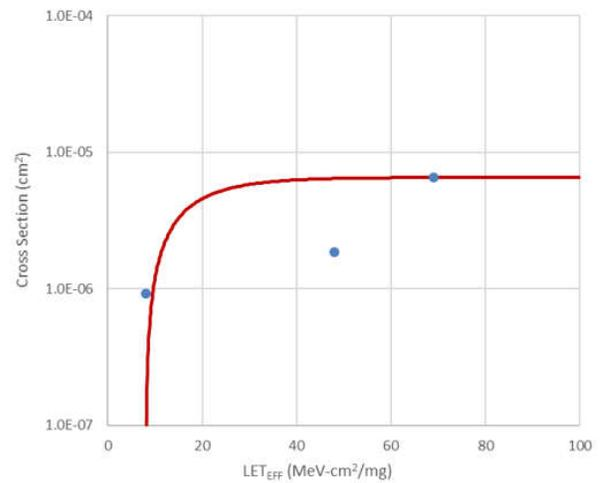
**Figure 3-23. Weibull Plot: V+ 1.7 V - Channel 6**
