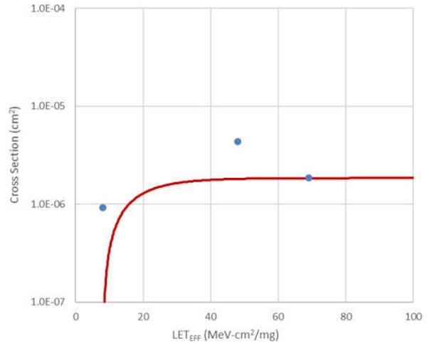
**Figure 3-15. Weibull Plot: V+ 1.7 V - Channel 2**
