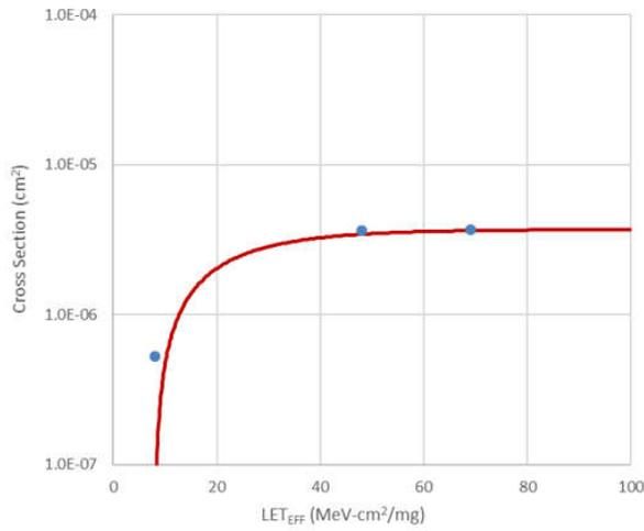
**Figure 3-22. Weibull Plot: V+ 2.0 V - Channel 5**
