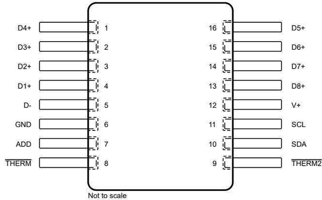
**Figure 2-2. TMP9R00-SP HKT Package 16-Pin CFP Top View**
