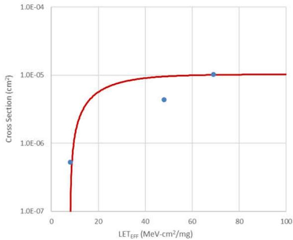
**Figure 3-18. Weibull Plot: V+ 2.0 V - Channel 3**
