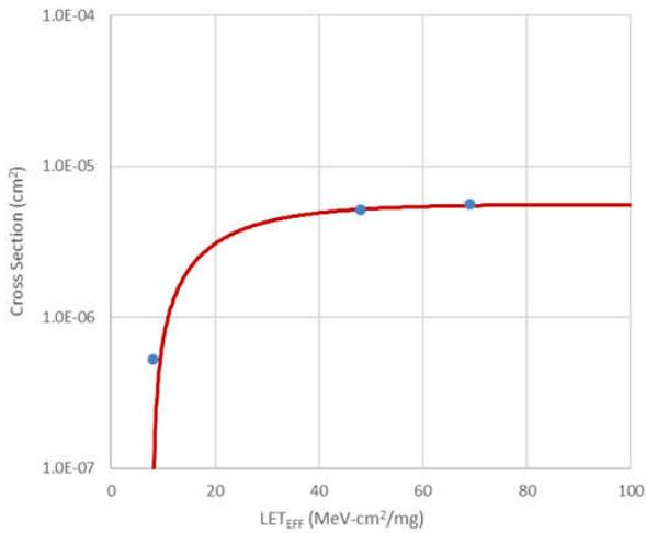
**Figure 3-14. Weibull Plot: V+ 2.0 V - Channel 1**
