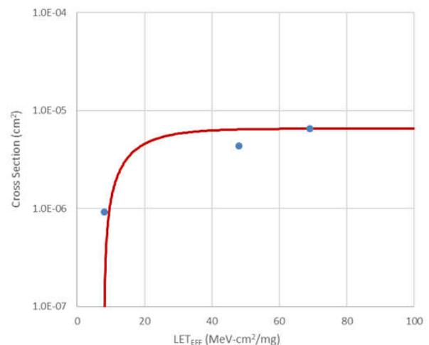
**Figure 3-19. Weibull Plot: V+ 1.7 V - Channel 4**
