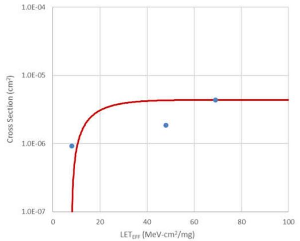
**Figure 3-17. Weibull Plot: V+ 1.7 V - Channel 3**
