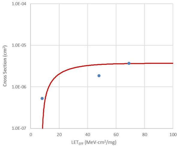
Figure 3-12. Weibull Plot: V+ 2.0 V - Local Channel
