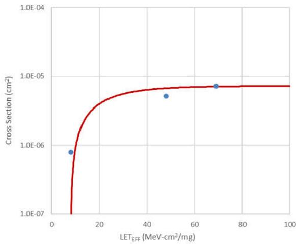
Figure 3-26. Weibull Plot: V+ 2.0 V - Channel 7
