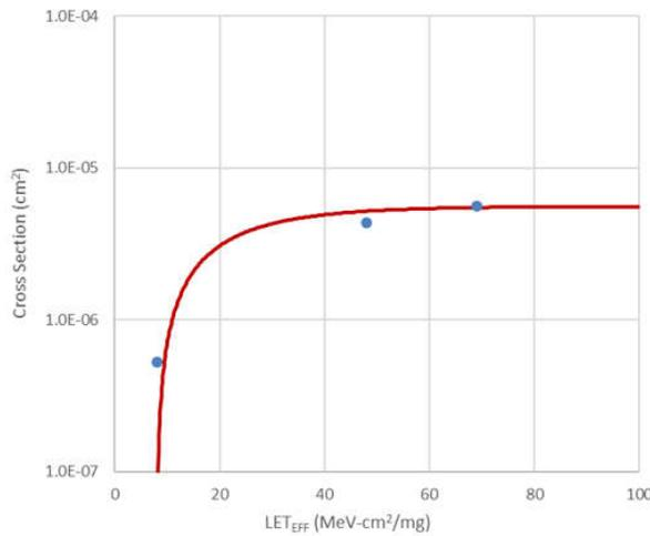
**Figure 3-24. Weibull Plot: V+ 2.0 V - Channel 6**
