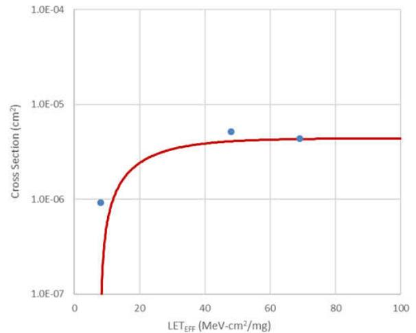
Figure 3-13. Weibull Plot: V+ 1.7 V - Channel 1
