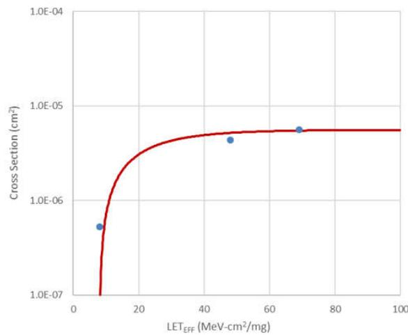
Figure 3-28. Weibull Plot: V+ 2.0 V - Channel 8
