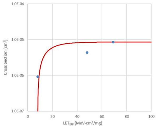
Figure 3-27. Weibull Plot: V+ 1.7 V - Channel 8
