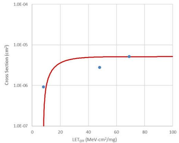
**Figure 3-25. Weibull Plot: V+ 1.7 V - Channel 7**
