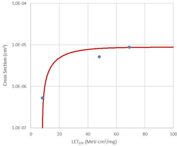
**Figure 3-20. Weibull Plot: V+ 2.0 V - Channel 4**
