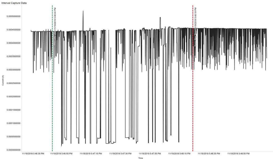
**Figure 3-1. Current vs Time for V<sub>CC</sub> Supply During SEL Run #2**
