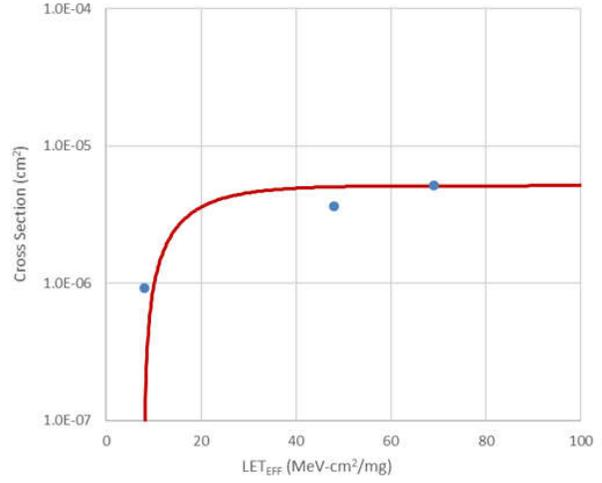
**Figure 3-21. Weibull Plot: V+ 1.7 V - Channel 5**
