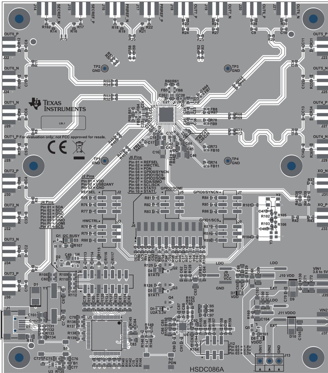
Figure 11. Top Layer Composite View
