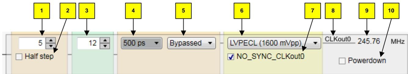
**Figure 2. Clock Outputs Page CLKout Path Description Diagram**
