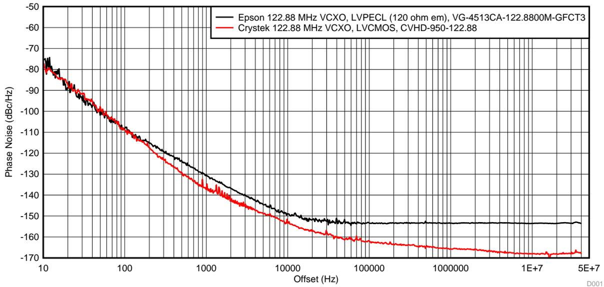
Figure 18. VCXO Phase Noise at 122.88 MHz
