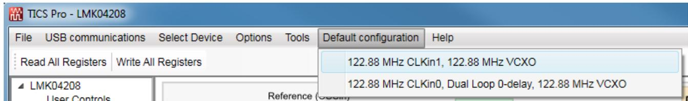
Figure 4. Setting the Default Mode for LMK04208
