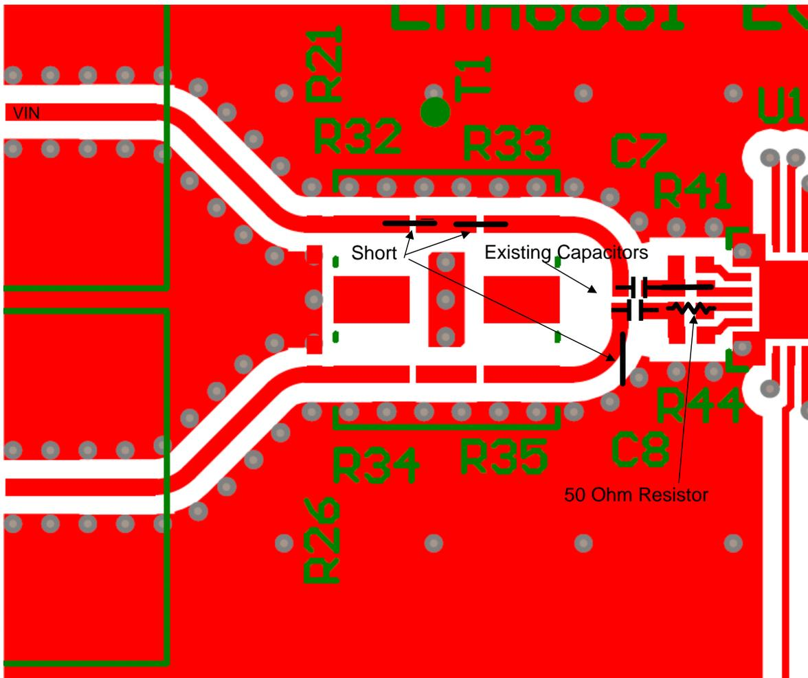
Figure 4. Input Configuration for Single Ended Signal. R44 should be 50Ω to ground. R32, 33 are 0Ω shorts. R34 and R35 are not needed.
