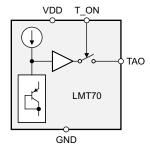
Figure 8. Simplified Block Diagram
