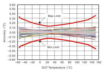
Figure 10. LMT70 Accuracy Over Temperature
