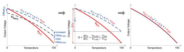
Figure 12. Two-Point Calibration Requires Offset Adjustment (left), Gain Adjustment (middle) to Yield the Final Transfer Function (right)
