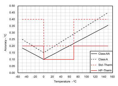
Figure 4. Accuracy Comparison Between Precision RTDs and Standard and Precision Thermistors
