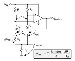
Figure 6. V<sub>PTAT</sub> Temperature Sensor
