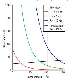
Figure 3. R-T Curve Comparison Between Thermistors and RTD
