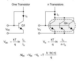
Figure 5. Principle of Eliminating I<sub>c</sub> and I<sub>s</sub>
