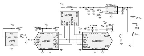
Figure 14. High Precision Temperature Transmitter With 4-to-20 mA Output
