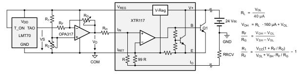
Figure 15. Low-Cost Temperature Transmitter With 4-to-20 mA Output
