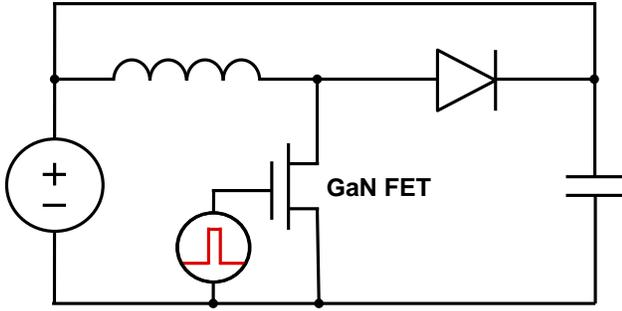
Figure 6: Schematic of the inductive hard-switching test vehicle
