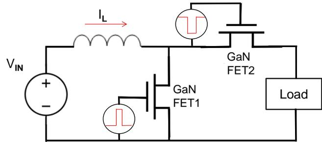
Figure 2: Boost-converter schematic
