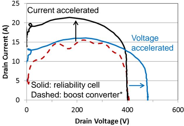
Figure 7: I-V locus showing voltage and current acceleration capability. The boost converter is simulated and the reliability cell data is measured.
