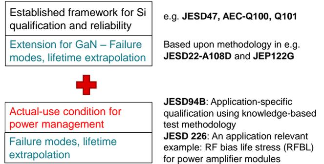
Figure 1: Qualification framework for GaN, built upon JEDEC documentation. The silicon framework is extended for GaN-specific failure modes and application-relevant testing is added.
