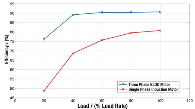
Figure 12: Efficiency comparison\*
