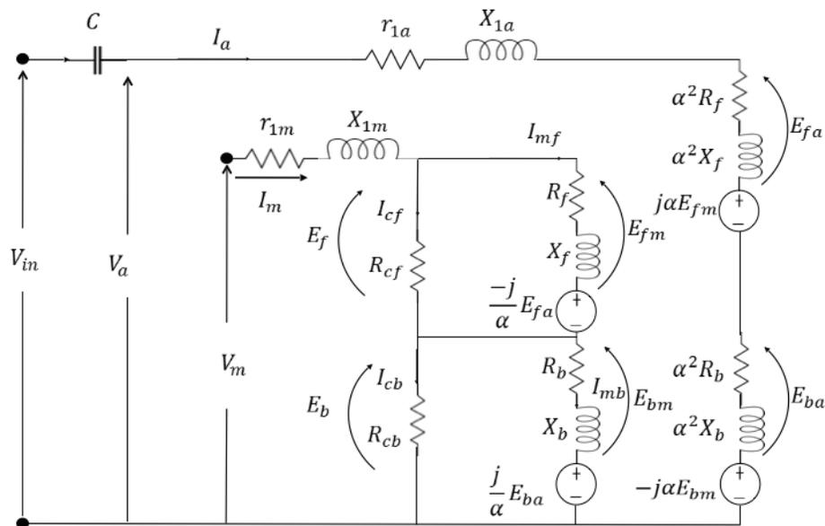
Figure 4: Equivalent circuit model for a SPIM [3]
