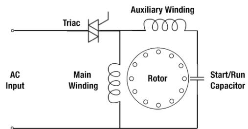
Figure 3: Capacitor start/run single-phase induction motor drive [1]
