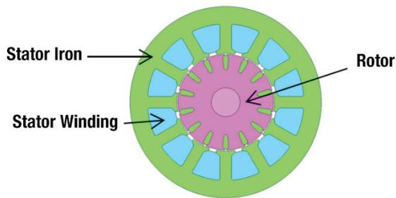
Figure 2: Single-phase induction motor example cross section
