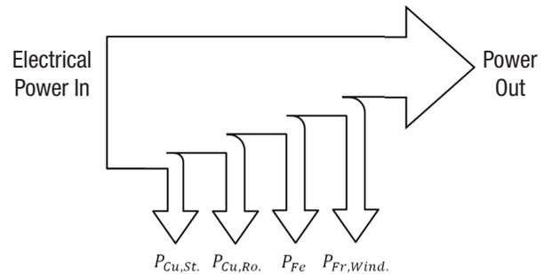
Figure 6: Losses in a single-phase induction motor [02]
