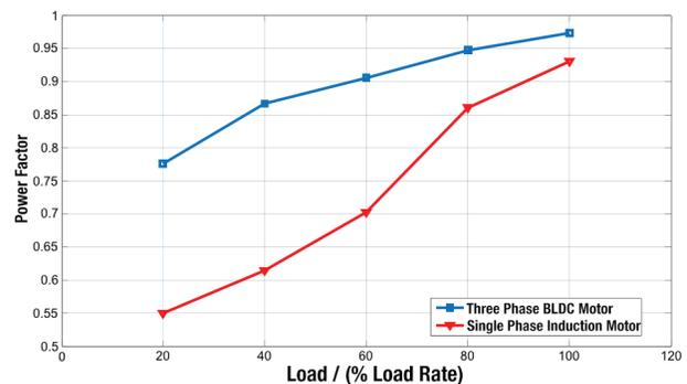
Figure 13: Power factor comparison\*
