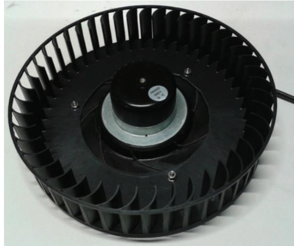
Figure 14: Three-phase BLDC motor with fan blades used in the experiment
