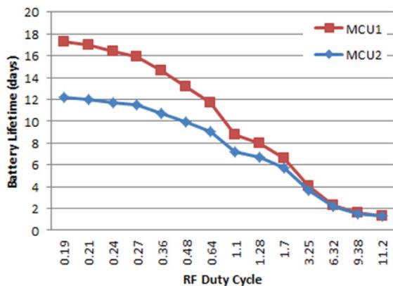
Figure 3. Simulated battery lifetime as a function of RF duty cycle.
