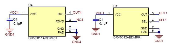
Figure 2. DRV5011 Coupon Board Schematic
