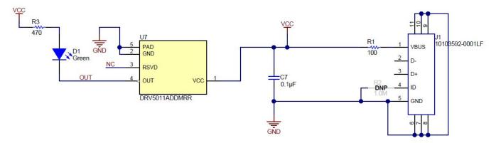
Figure 1. DRV5011 Center Board Schematic
