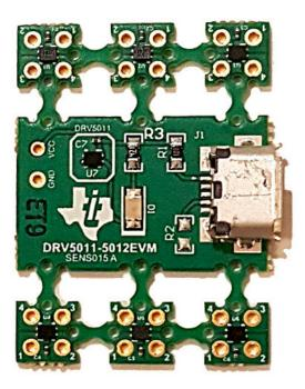
This user's guide describes the characteristics, operation, and use of the DRV5011-5012EVM evaluation module (EVM). This EVM is designed to evaluate the performance of the DRV5011 and DRV5012 ultralow power digital-latch Hall effect sensors. Throughout this document, the terms evaluation board, evaluation module, and EVM are synonymous with the DRV5011-5012EVM. This document includes a schematic, reference printed-circuit board (PCB) layouts, and a complete bill of materials.
