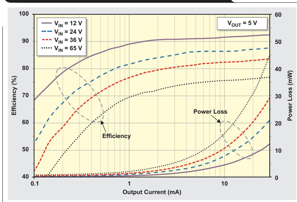
The total current budget must be sufficient to power all functional blocks of the transmitter: sensor interface and excitation, linearization method (MCU), galvanic barrier jump (if needed), 4–20-mA loop driver, and so forth. The solution presented was an integrated and robust DC/DC buck converter that has ultra-high efficiency across wide supply-voltage and load-current ranges. The resulting compact solution was achieved with minimal design effort.
