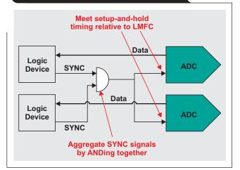
SYNC signal in that it must meet the needed setup-andhold times relative to the LMFC edge in the transmitting device. If DDCs or DUCs are not used in the ADCs or DACs, then there is no requirement for SYNC signal timing and each device can start up at independent times and still achieve synchronization.
