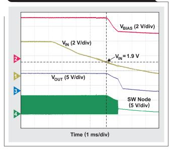
split-rail approach feeding  $V_{\rm OUT}$  back as the bias supply works. A separate bias supply different from the battery input is needed.
