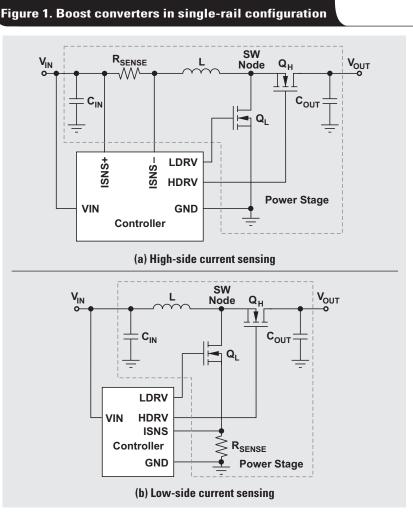
comparator. Therefore, it is not required to match the minimum common-mode voltage. Consequently, in the single-rail configuration where the input voltage to the power stage and the bias voltage to the controller are tied together, the controller's input UVLO threshold imposes a constraint on how low the input voltage to the boost power stage can go.
