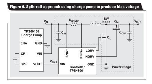
to the battery (Figure 2). If not, a charge pump can be added for a bias supply (Figure 6).
