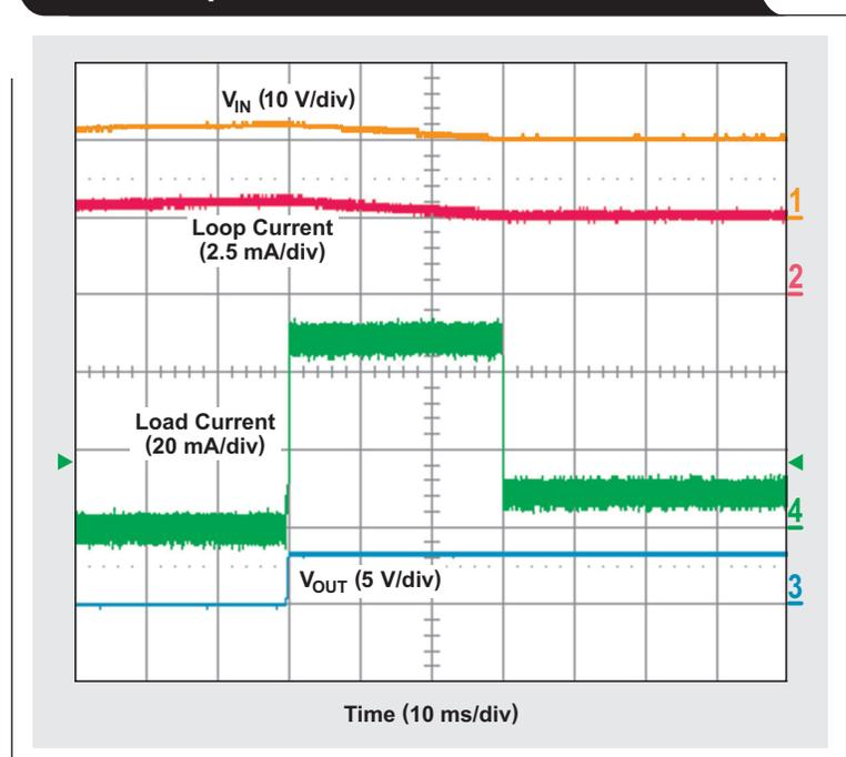
Finally, the energy-harnessing power supply stores enough energy in the bulk capacitor and operates over a wide enough input-voltage range to supply continuous pulses of power to the load. Figure 5 shows the supply providing 20 mA to the load for a duration of 100 ms every second, with the supply's output voltage remaining regulated.
