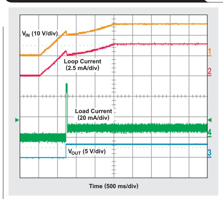
**Figure 4. Energy-harnessing power supply providing load's start-up current**
