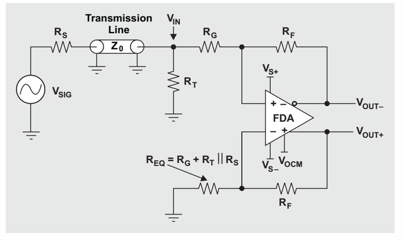
**Figure 7. Positive side of FDA circuit**
