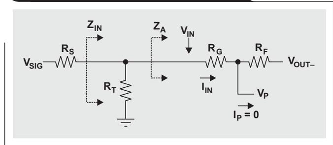
**Figure 8. Thevenin equivalent of positive side**
