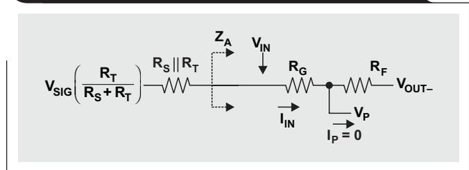
equation for only the amplifier's AC or signal response to  $V_{OUT-}$ , which we will call  $V_{OUT- (AC \text{ only})}$ :
