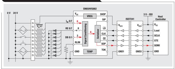
The designer can further reduce the number of external components by using the integrated debounce filter, set to filter pulses of less than 3 ms or 1 ms in duration. For the fastest acquisition of glitch-free switches, bypass the filter as well.
